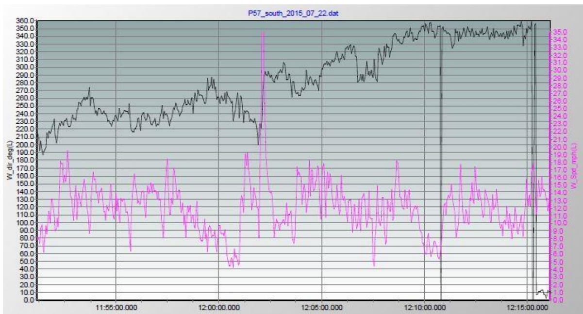
Figure 21. Wind speed and wind direction values collected at three-second intervals between 11:50h and 12:15h (PST) on June 14, 2015.
