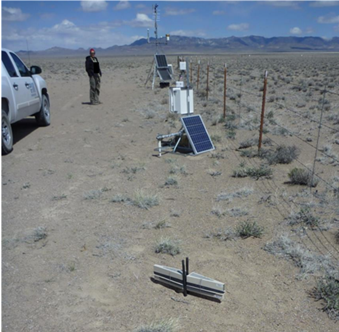
Figure 24. Photos of the BSNE saltation sand trap installations at Project 57 are not available. However, this photograph taken at Clean Slate III on the Tonopah Test Range (Nikolich, 2016) shows a typical installation, which is essentially identical to the Project 57 installations. The BSNE saltation sand trap in the foreground is oriented with one opening facing the dominant wind direction coming across the Contamination Area, which is to the right of the fence, and one facing away from the Contamination Area.
