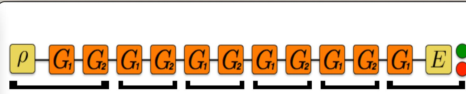
**A typical GST experiment.** A “germ” -- one of several short sequences designed to single out particular parameters -- is repeated many times to amplify errors, and bookended by short “fiducial” sequences.
