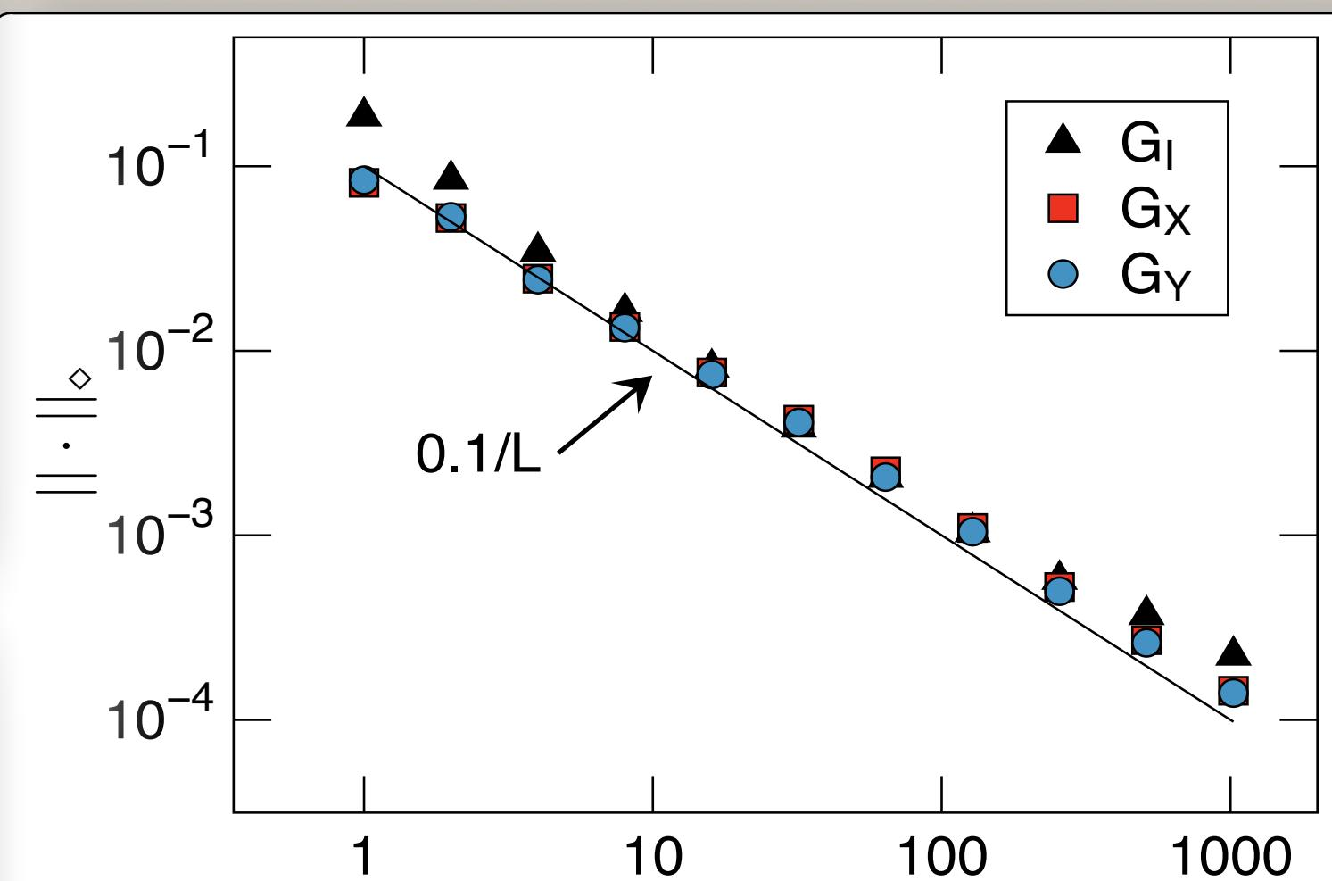
**GST estimation error (diamond norm) scaling.** Simulated GST (with assorted known true gates), shows Heisenberg scaling: The diamond norm error scales as  $1/L$  with max. sequence length
