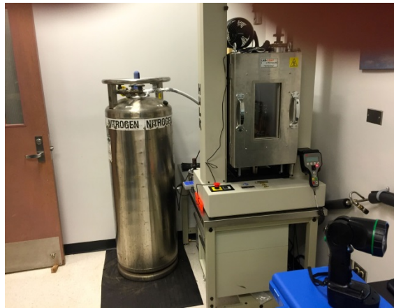
Figure 9. Therm-Craft Lab-Temp chamber with 180 liter liquid nitrogen dewar. Up to three different capillary rheometers were placed in the chamber for measurements at any one time.
