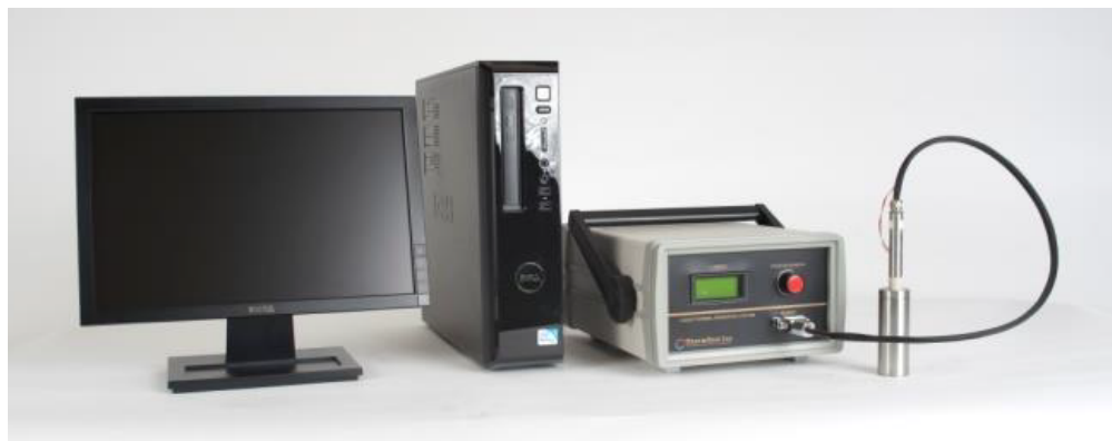
Figure 18. ThermTest transient hot wire apparatus showing sample holder on the right.
