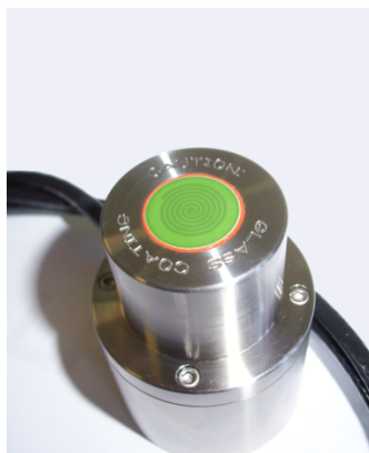
Figure 17. Left: TCI thermal conductivity analyzer showing coil. Right: Thermal conductivity of water measured with both the TCI and THW probes. The literature value is within the stated \pm 5\% uncertainty for both apparatuses.
