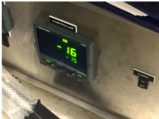
Figure 10. Temperature control unit where the set temperature is shown left and the temperature measured by the thermocouples built into the chamber are displayed right. The chamber temperature can fluctuate as much as \pm 2 °C as the evaporated nitrogen is blown into the chamber. The platinum resistance thermometer is immersed in a beaker of PDMS fluid with approximately the same volume as that held in the capillary rheometers.
