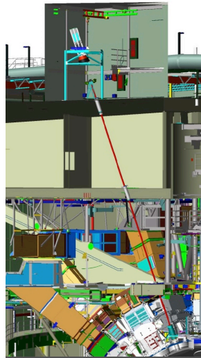
Figure 1. LOS layout. Primary neutron beam is the red line and terminates on the detector.
