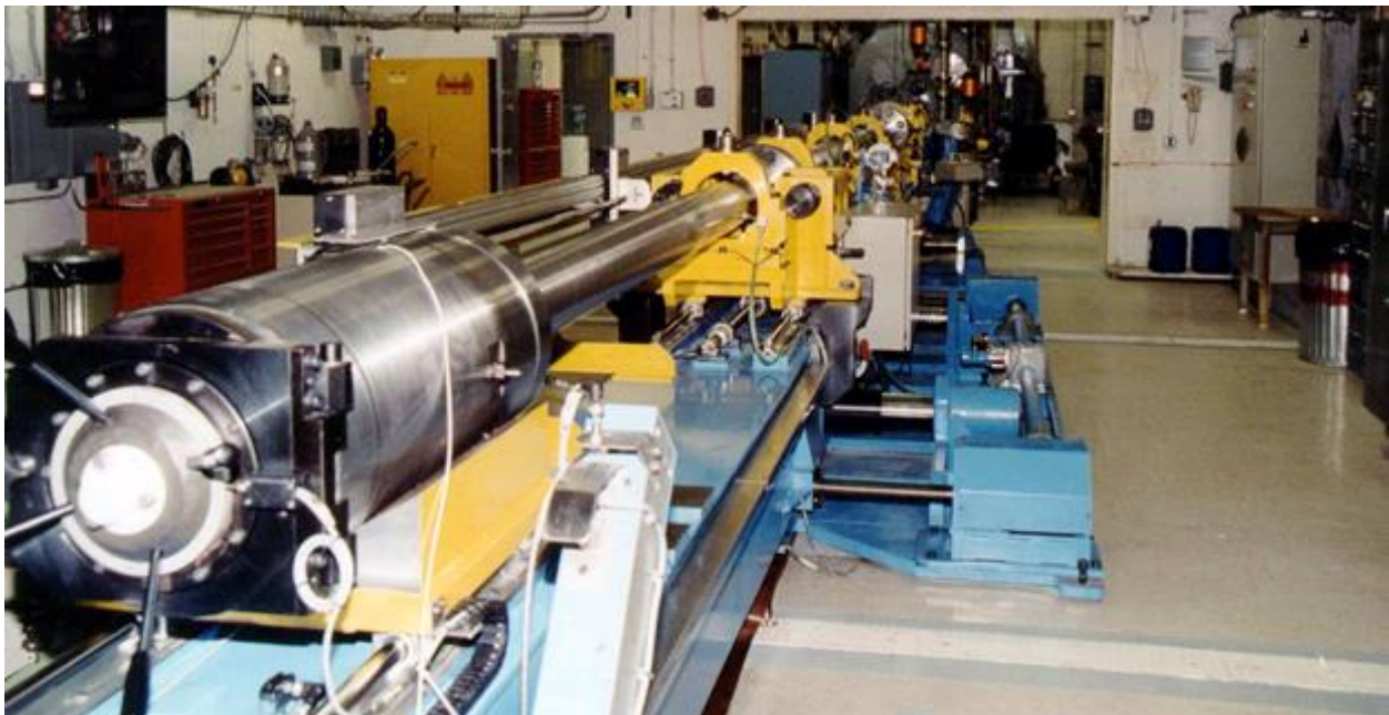
Figure 1: The Jasper two-stage gas gun at the Nevada National Security Site, as seen from the loading port. The target chamber is visible in the background.
