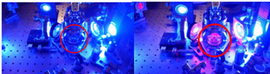
Fig. 6. Marked quenching of fluorescence from Ti:sapphire pumped with with high-power 450 nm diodes. Left: 50W input power, Ti:sapphire crystal at 295 K. Note that the cryocell window is dark. Right: same, but crystal at 93 K. Note that this behavior is not as marked with 532 nm pumping, suggesting new gain dynamics in the system.
