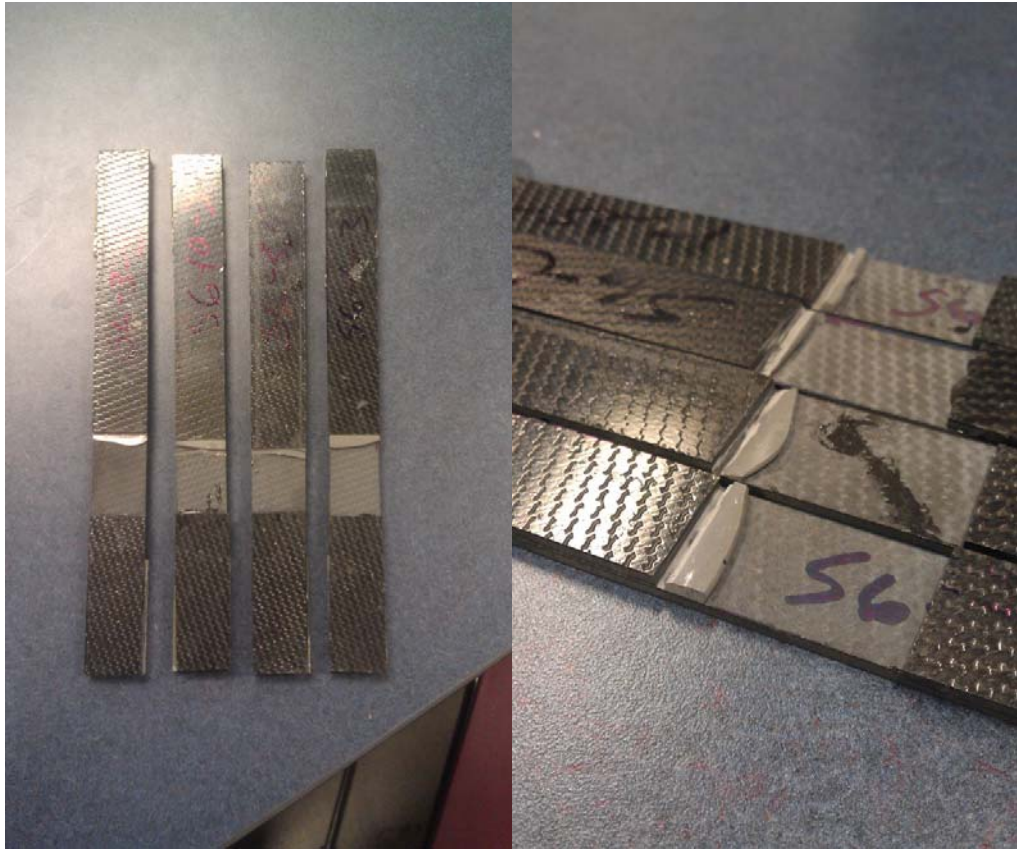
Figure 5.1 Optical image showing the geometric details of a SSL specimen.
