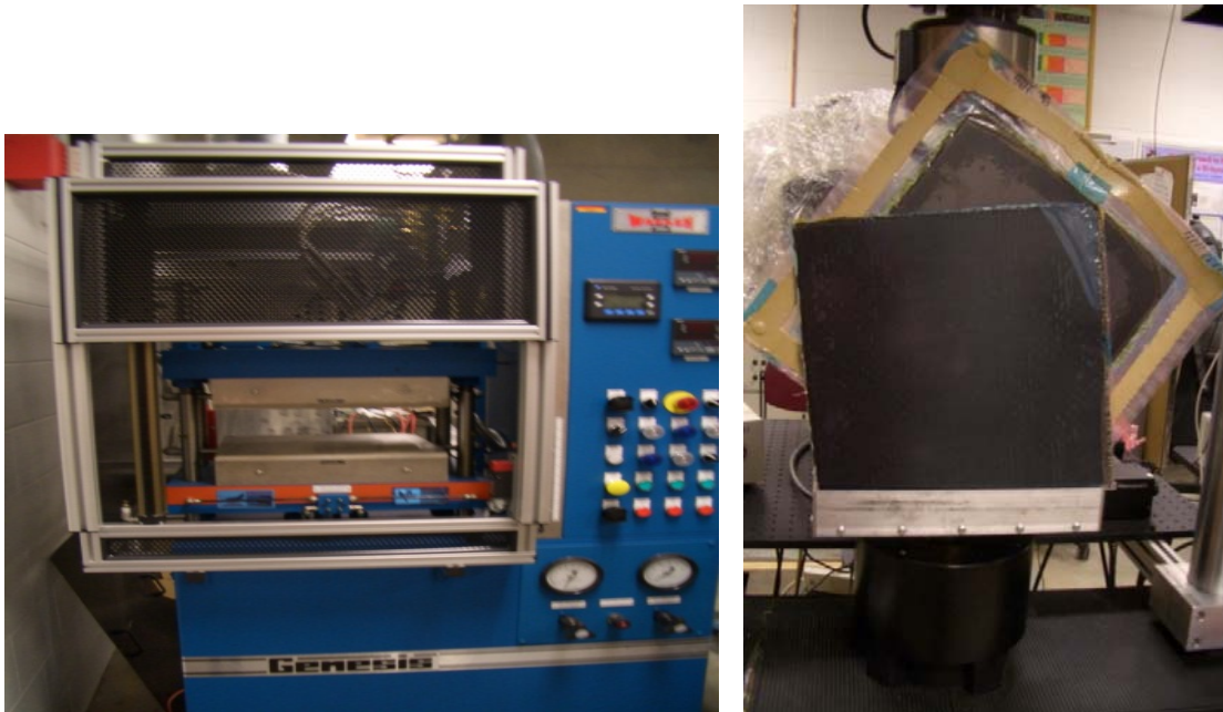
Figure 2.2 (a) The hot-press for laminate manufacturing; (b) A typical composite laminate
