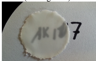
Figure 8. Picture of PDMS/PMMA-alumina composite film (film thickness = 0.3 mm). Particle aggregation results in significant scattering losses.
