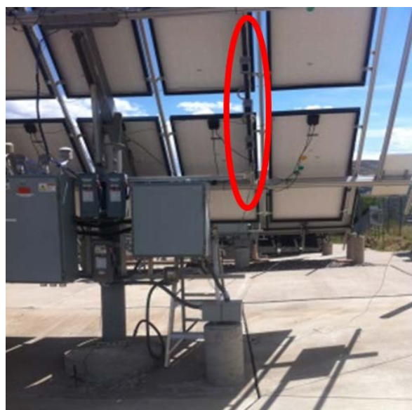
Fig. 1. Back surface irradiance measurement locations on the NREL array.
