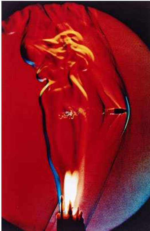
Schlieren photograph of a bullet passing through a candle flame. Edgerton and Vandiver, 1973.
