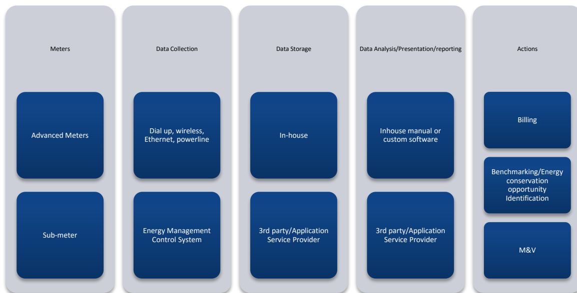
Figure 3.1: Schematic Showing an Advanced Metering System
