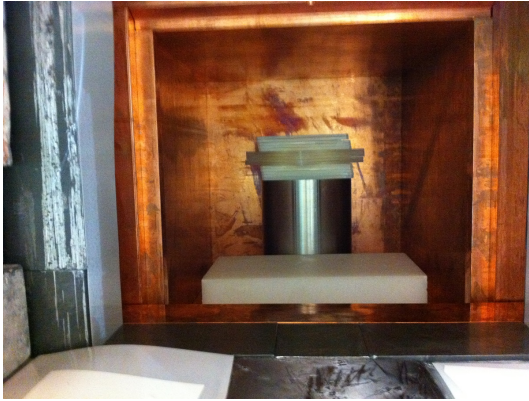
Figure 8.4: Zytel nylon (Zytel 101 NC010 Nylon 6,6 Polyamide) sample (stack of white squares) in the Gopher screening cavity. The white brick in front is polyethylene, which is left in the cavity since it was present in the background spectrum run.
