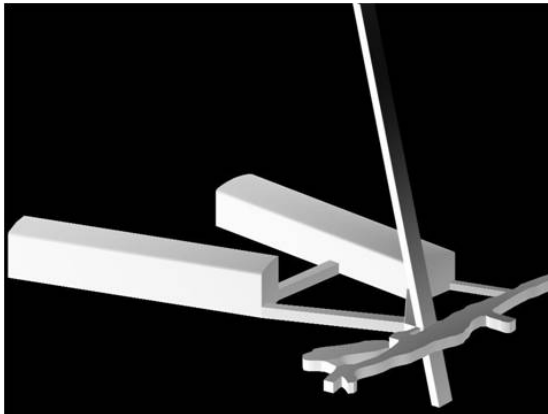
Figure 5.1: Computer rendering of the Soudan Underground Laboratory. White indicates open space while black indicates rock. The Soudan 2 and MINOS caverns are the large rectangular blocks on the right and left respectively. They are connected to each other and the historical tunnels by small access tunnels. The historical drift is the rough-edged tunnel which leads off to the right. The angled vertical tunnel is the shaft to the surface. The CDMS experiments were housed in the Soudan 2 cavern.
