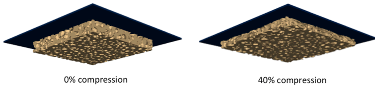
Figure 6. Finite element modeling of a CT foam sample under uniaxial compression.
