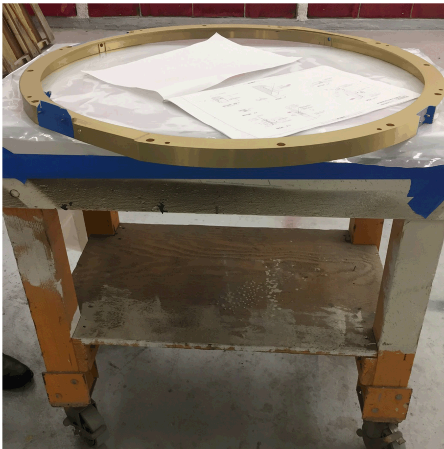
Figure 2: Image of filter frame on preparation cart showing nature of paint shop cleanliness. The paint shop by it's nature is a non-clean envirmnt with high level of airborne particulate.
