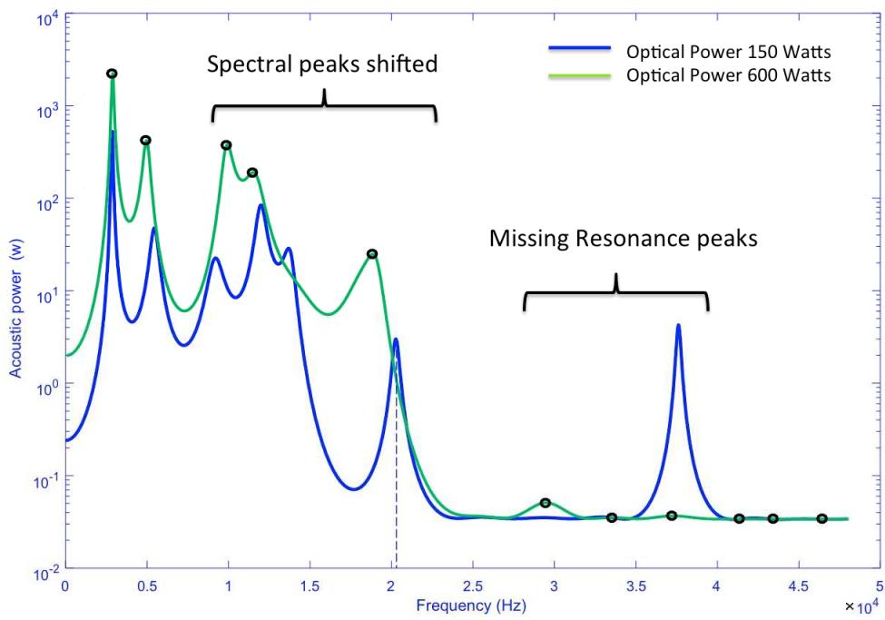
**Figure 1.0.** The graph compares the average acoustic spectra from 50 scans signal for each of the two optical power settings. The data clearly shows that resonance peaks are shifted, or in some cases, completely missing depending on the incident optical power. This measurement represents an encouraging first step towards further application of acoustic signals as a diagnostic parameter for SLM process monitoring.
