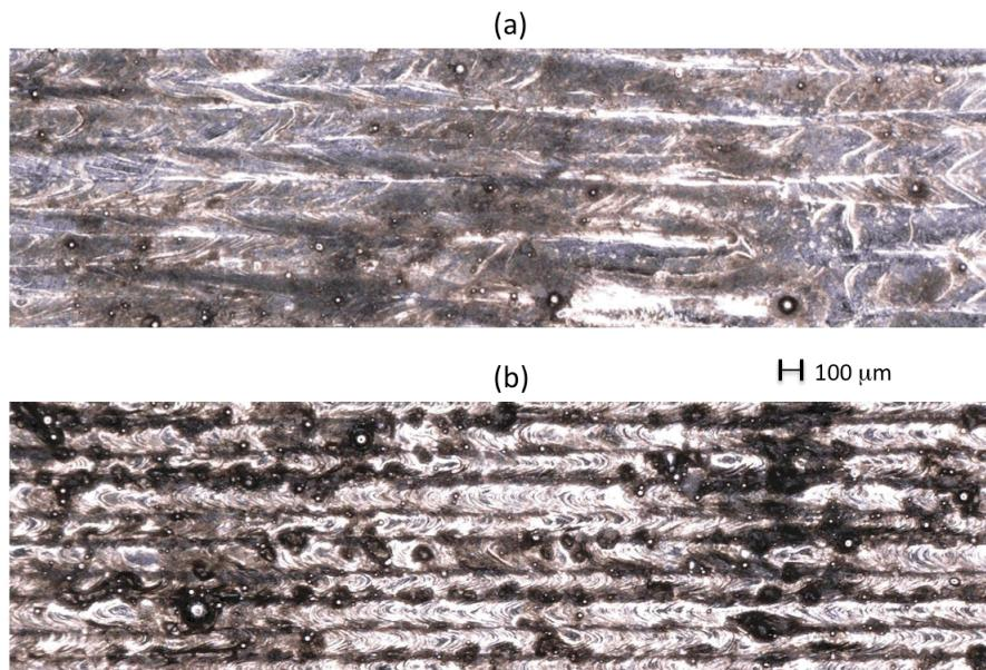
**Figure 2.0.** Microscope image showing the SLM traces on the surface of the build plate for the two incident optical powers; (a) 600 Watts, and (b) 150 Watts. The laser scan velocity was constant at 250 mm/sec for both sets of traces.
