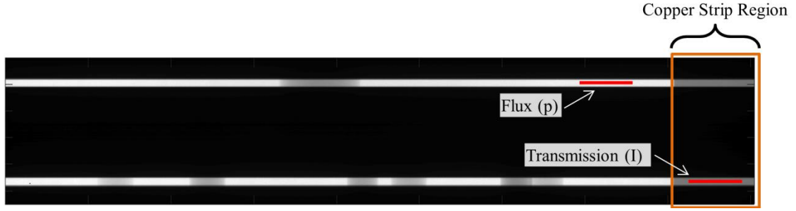
Figure 9 Sample raw radiograph illustrating location of parameters used to calculate the Cu strip metric.
