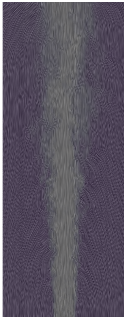
Figure B.6. Visualization of a 2D slices through the center of the 3D lifted ethylene jet flame. Lighter color represents faster velocity.
