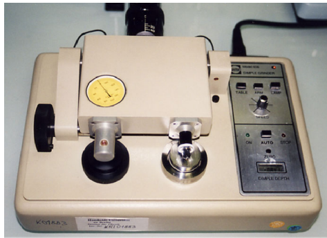
Figure 8 Gatan Dimpler for pre-thinning a TEM disc Prior to ion milling.
