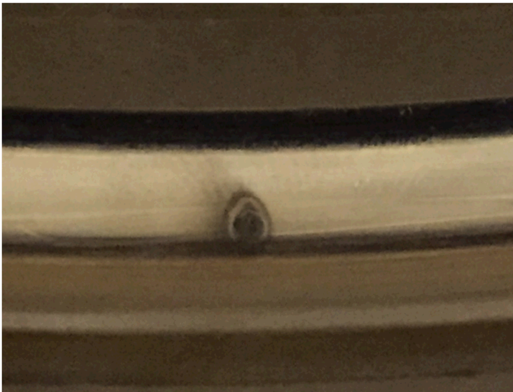
Figure 1: Arcing on the RV's support bearings.
