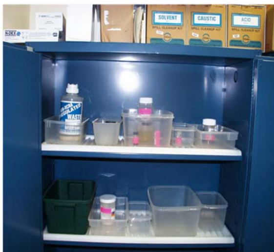
Satellite accumulation area.
