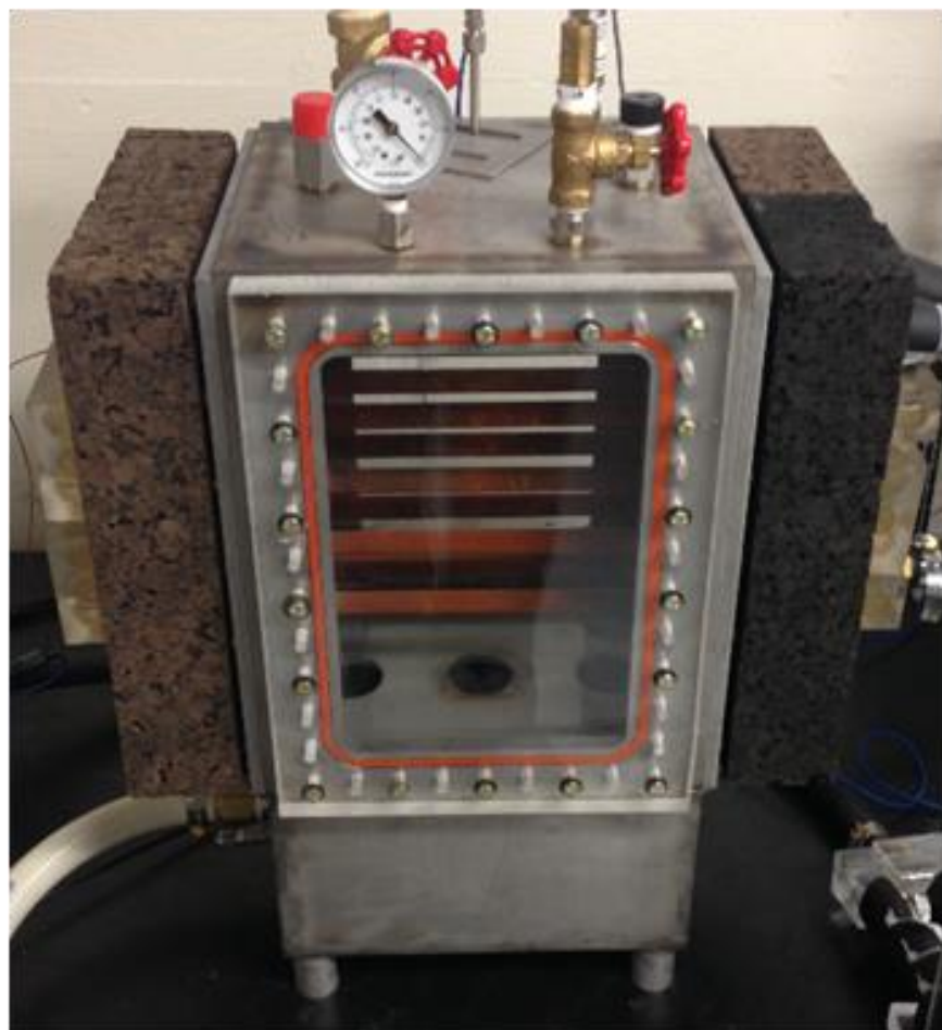
Figure 5-43. Photo of the final stainless steel, horizontal-tube, falling-film heat exchanger.
