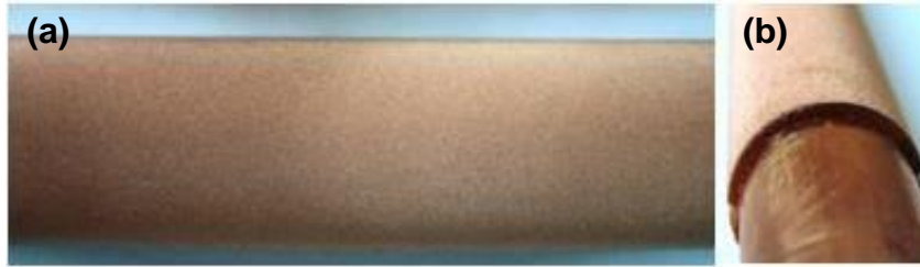
Figure 5-1. (a) Photograph of the porous-layer coated tube showing (b) the porous coating (1 mm thick) of sintered copper particles (75 \mu\text{m} in diameter).
