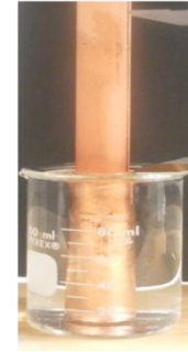
Figure 5-2. Wicking height measurement for pore diameter estimation.
