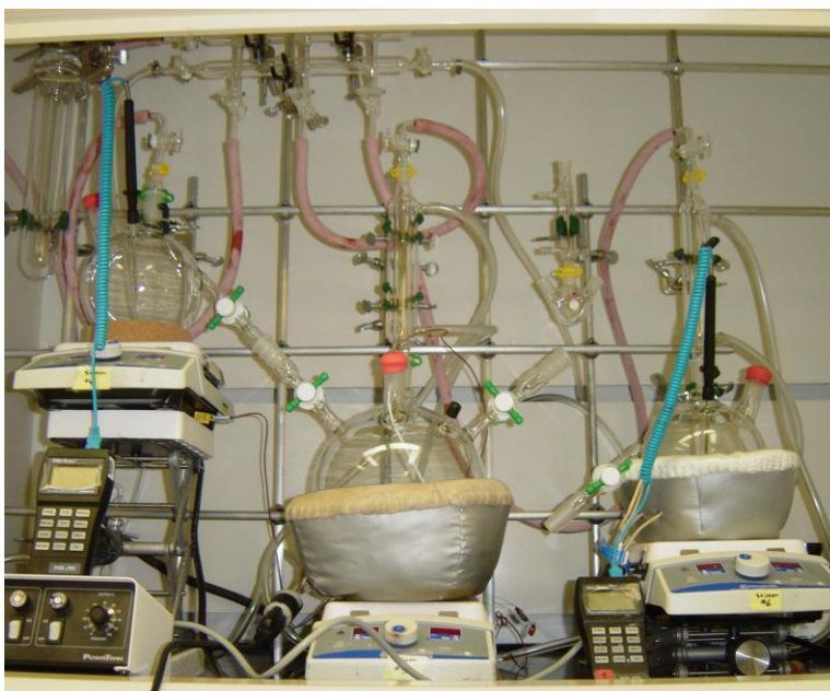
Figure 6. Photograph of high-reaction-volume synthesis set-up for up-scaled quantum dot production.
