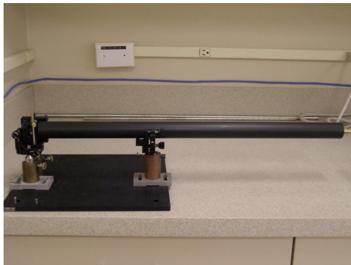
Figure 12. Mock tool on bench in 24" long 1.18" diameter tube.
