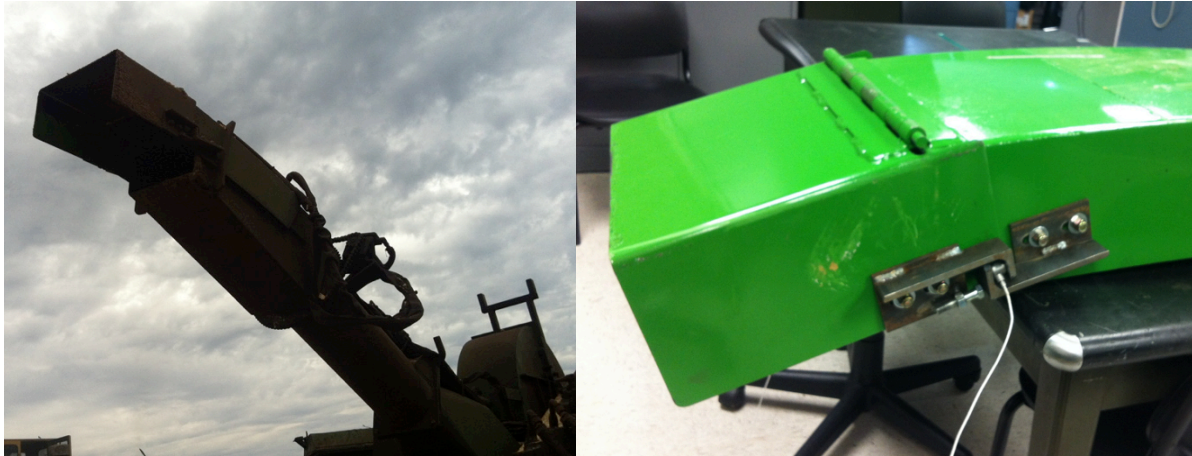
Figure 8.2.9 The mass flow sensor (including force transducer) mounted on the chipper (left) and a close-up photo (right) showing the mechanism used to transmit impact force from the hinged plate to the transducer.
