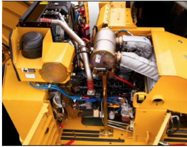
Painless maintenance routines. Excellent access to both sides of the engine and all daily service points through the swing-out doors. Hydraulic pumps are housed in a compartment separate from the engine.
