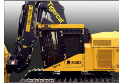
Painless maintenance routines. Excellent access to both sides of the engine and all daily service points through the swing-out doors. Hydraulic pumps are housed in a compartment separate from the engine.
