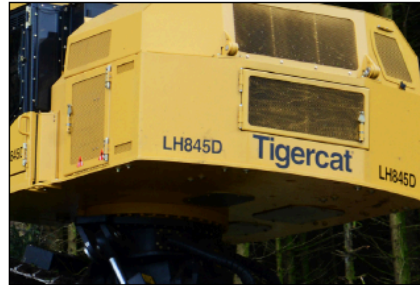
Rear intake is well away from the saw discharge area.
