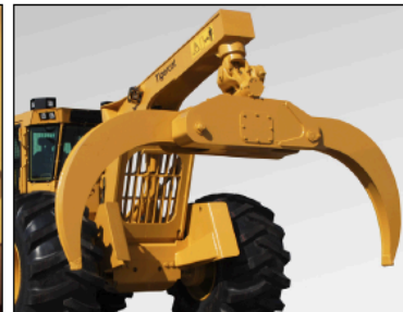
High capacity dual cylinder grapples and high visibility arch
