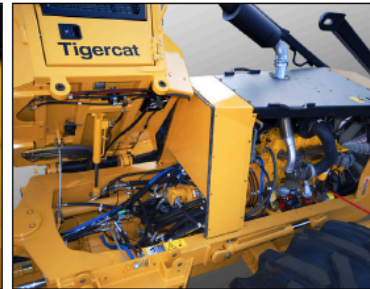
Tilting cab to access pumps and driveline
