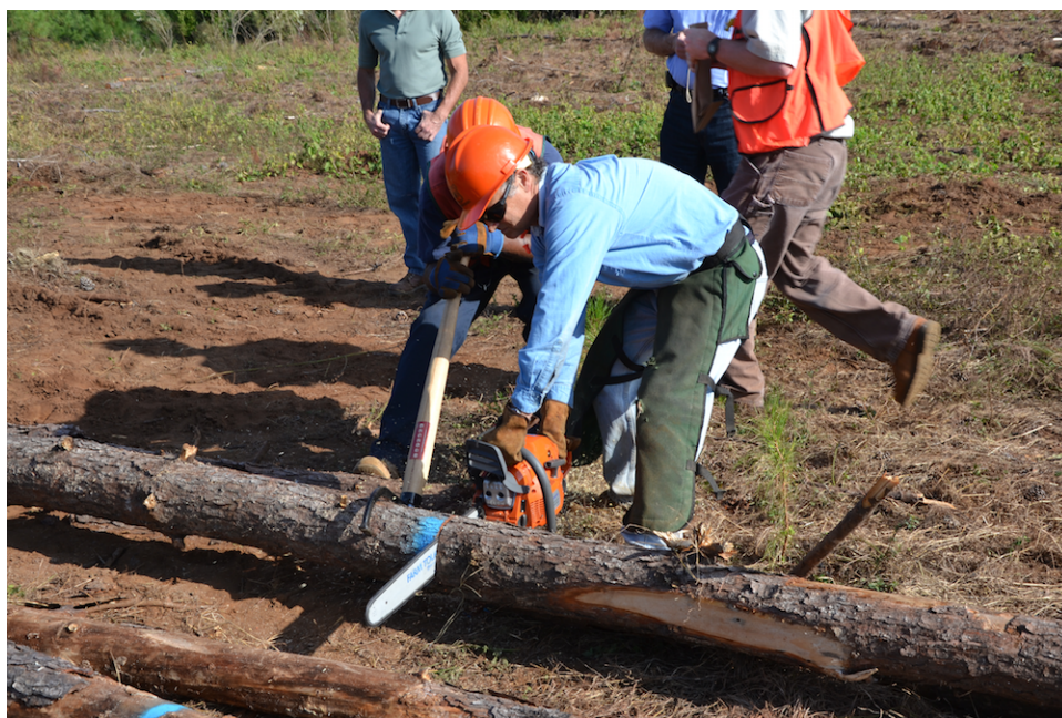
Figure 8.7.4 Example of collecting disks from trees for moisture content determination.
