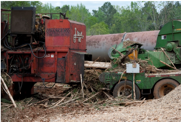
Figure 8.9.6. The air sampler was placed near the throat of the chipper.
