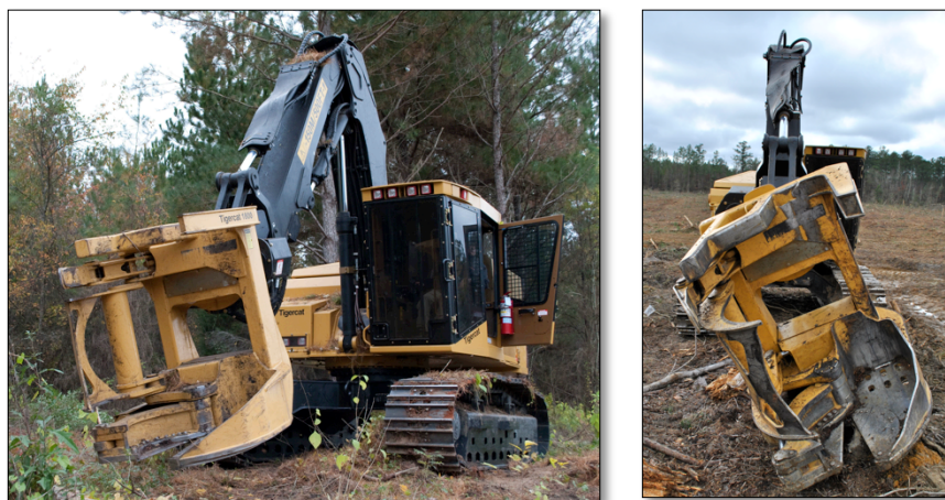
Figure 2.6 DT1802 high-speed shear felling head illustrating the ability to rotate the head with the 340 degree rotation wrist.
