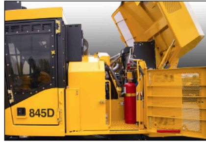
Painless maintenance routines. Excellent access to both sides of the engine and all daily service points through the swing-out doors. Hydraulic pumps are housed in a compartment separate from the engine.
