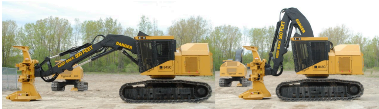
Figure 2.5 ER ® technology boom system allows planar movement of the boom system (both main boom and stick boom) through a single joystick movement.
