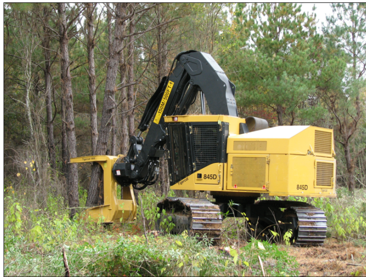
Figure 2.3 Tigercat 845D Biomass Harvester shown in renderings during the design phase and in the field as the final prototype machine.
