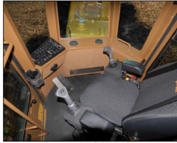
Turnaround™ provides full rear facing drive controls
