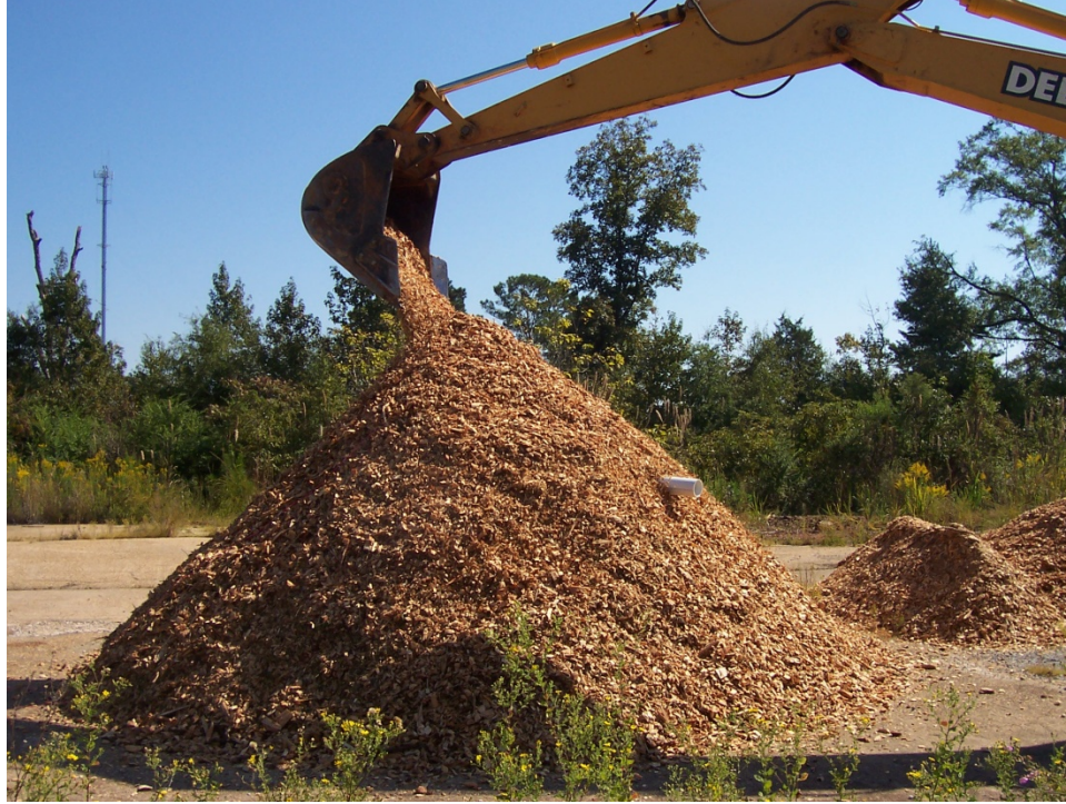
Figure 7.1 Chip pile construction using an excavator.
