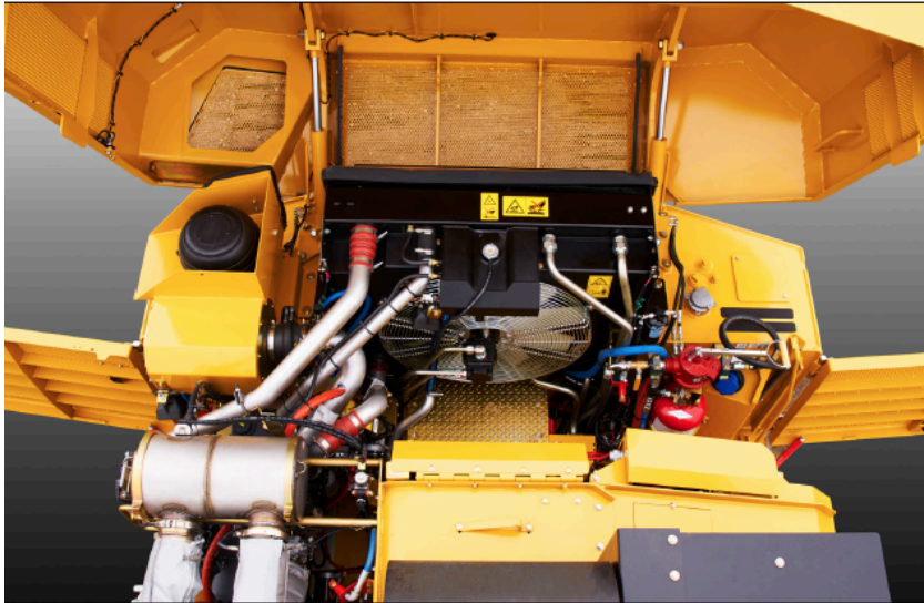
Clamshell-style engine enclosure for full, easy access to all major components including the engine, cooling system and valves. Neat hose and electrical routings.
