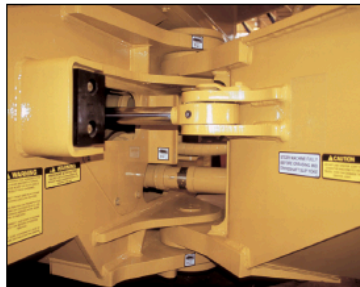
Strong centre section with large pins and tapered roller bearings
