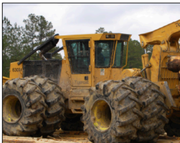
All D-series models are standard equipped for dual or flotation tires
