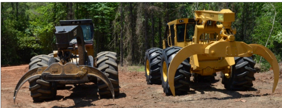
Figure 2.8. Visual comparison of the Tigercat 630D skidder (on right) with the 25 sq. ft. grapple and the Caterpillar 525 skidder (on left).
