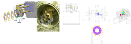
Figure 1: (left) Graphic depicting the target wheel and detector structure within the LENZ chamber, as well as photo of the physical LENZ chamber with the detectors assembled. (right) Image of Geant4 detector geometry, including closeup of the simulated S1 silicon detector.
