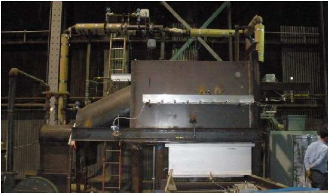
Figure 8: Large Batch Furnace – Front view (burner located on end of furnace at right).
