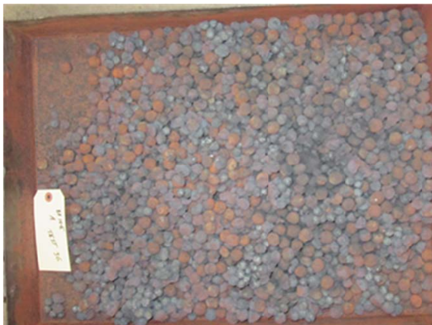
Figure 50. DRI produced at a furnace hot-zone temperature of 1500°C and residence time of 50 min. Dried greenballs which contain revert material (14-5) (molar C/O ratio = 1.1) were used as a feed material. The initial bed height of the dried greenballs was 7.6 cm. The DRI was cooled in the LHF cooler at a long residence time, and then was shoveled out to a tray and further cooled in nitrogen under the external hood.
