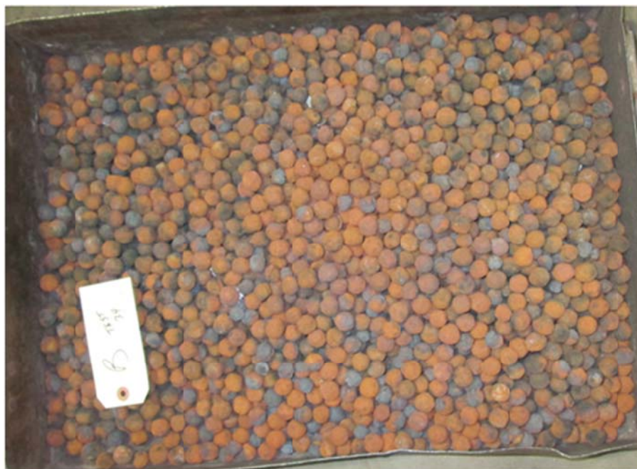
Figure 44. DRI produced at a furnace hot-zone temperature of 1400°C and residence time of 50 min. Dried greenballs which contain revert material (greenball recipe 14-5) (molar C/O ratio = 1.1) were used as a feed material. The initial bed height of the dried greenballs was 7.6 cm. The DRI was cooled in the LHF cooler at a long residence time, and then was shoveled out to a tray and further cooled in nitrogen under the external hood.
