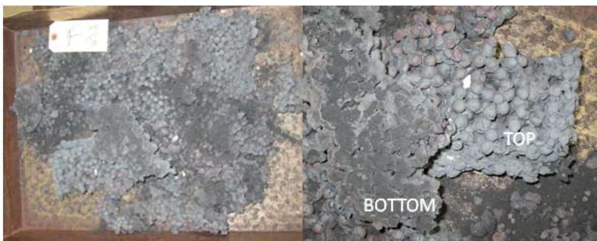
Figure 49. DRI produced at a furnace hot-zone temperature of 1450°C and residence time of 100 min. Dried greenballs which contain revert material (14-5) (molar C/O ratio = 1.1) were used as a feed material. The initial bed height of the dried greenballs was 7.6 cm. The DRI was cooled in the LHF cooler at a long residence time, and then was shoveled out to a tray and further cooled in nitrogen under the external hood.
