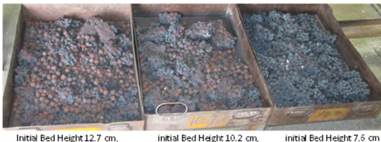
Figure 68 . DRI produced using dried greenballs which contain revert material (dried greenball recipe 14-8) (molar C/O ratio = 1.0) at a furnace temperature of 1500°C and residence time of 80 min at various initial bed heights. For these experiments, the DRI produced was cooled in the LHF cooler at a long residence time and shoveled into a tray and further cooled in nitrogen under the external hood.
