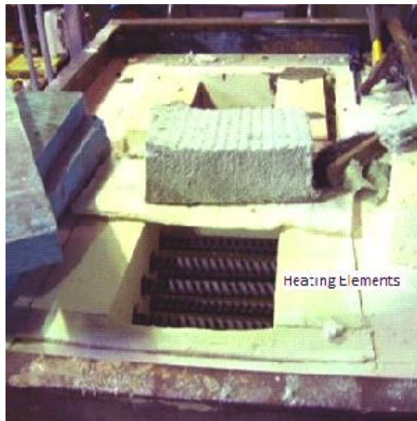
Figure 3: Top of Furnace and Heating Elements
