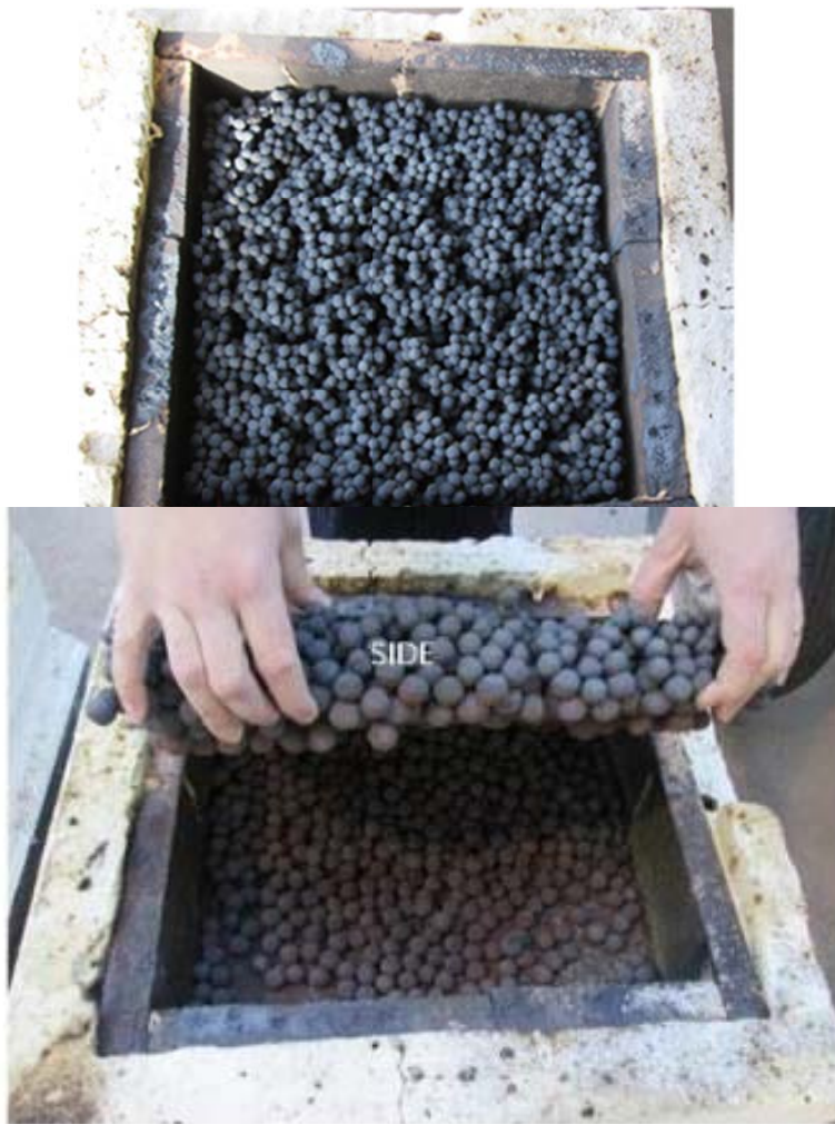
Figure 22. DRI produced using dried greenballs which contain magnetite concentrate (greenball recipe 13-1) (molar C/O ratio = 1.0) at an initial bed height of 12.7 cm, a furnace temperature of 1500°C, and a residence time of 80 min. The DRI was cooled in the LHF cooler (long residence time). A cart with sides of alumina brick was used for placing the dried greenballs in the LHF.
