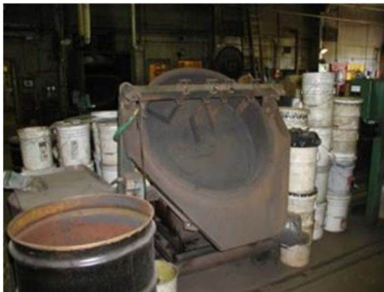
Figure 17. Pilot-scale balling disk 0.91 m (3 ft) diameter.
