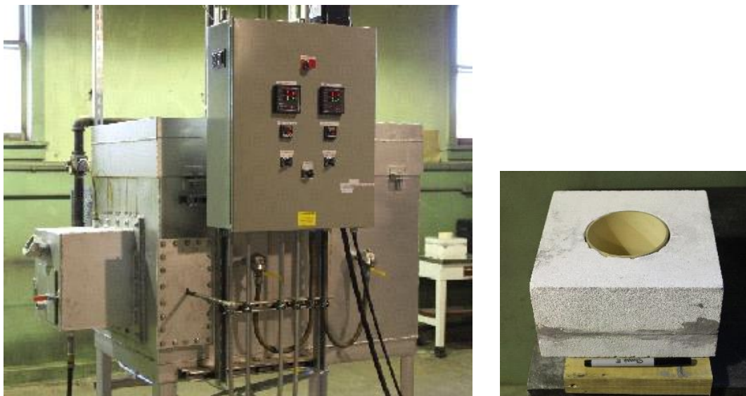
Figure 18. Two-zone, electrically heated laboratory furnace and insulated crucible used in tests for measuring kinetic factors.
