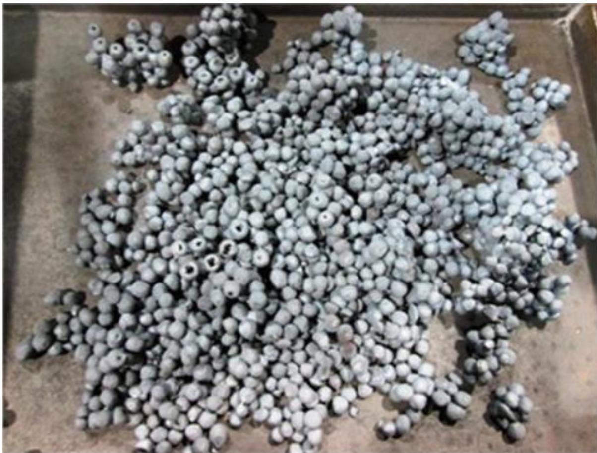
Figure 23. DRI produced at a furnace temperature of 1500°C and residence time of 80 min using dried greenballs which contain magnetite concentrate (greenball recipe 14-6) (molar C/O ratio = 1.1). DRI was cooled in the LHF cooler at a long residence time, and then it was shoveled into a tray and further cooled in nitrogen under the external hood. The bed height was 7.6 cm.
