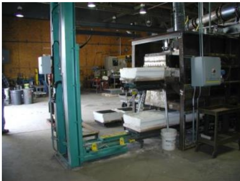
Figure 15. LHF moving cart system, discharge end.
