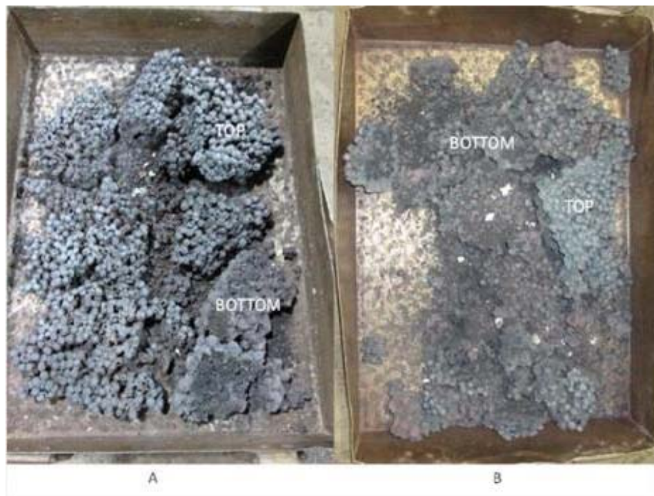
Figure 64 . DRI produced at a furnace hot-zone temperature of 1500°C and residence time of 80 min; the initial bed height was 7.6 cm. Sample A was produced using dried greenballs which had a molar carbon-to-oxygen ratio of 1.1 (greenball recipe 14-5), and sample B was produced using dried greenballs which had a molar carbon-to-oxygen ratio of 1.0 (greenball recipe 14-8). For these experiments, the DRI produced was cooled in the LHF cooler at a long residence time and then shoveled into a tray and further cooled in nitrogen under the external hood.
