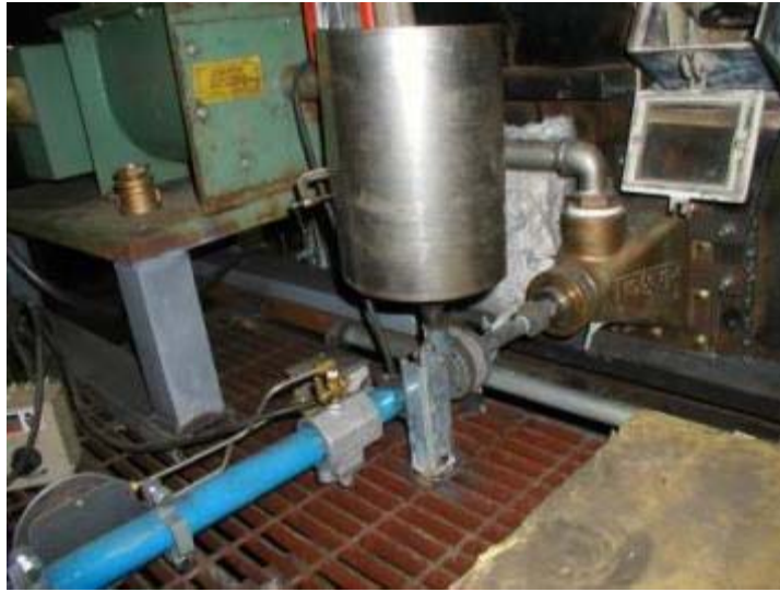
Figure 12. Oxy-coal burner, orifice plate and Eductor system.
