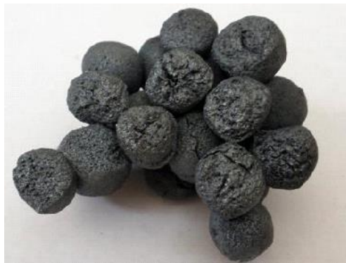
Figure 5. Cluster of pellets from early Large Batch Furnace Test with overheating/reoxidation of pellet surface.
