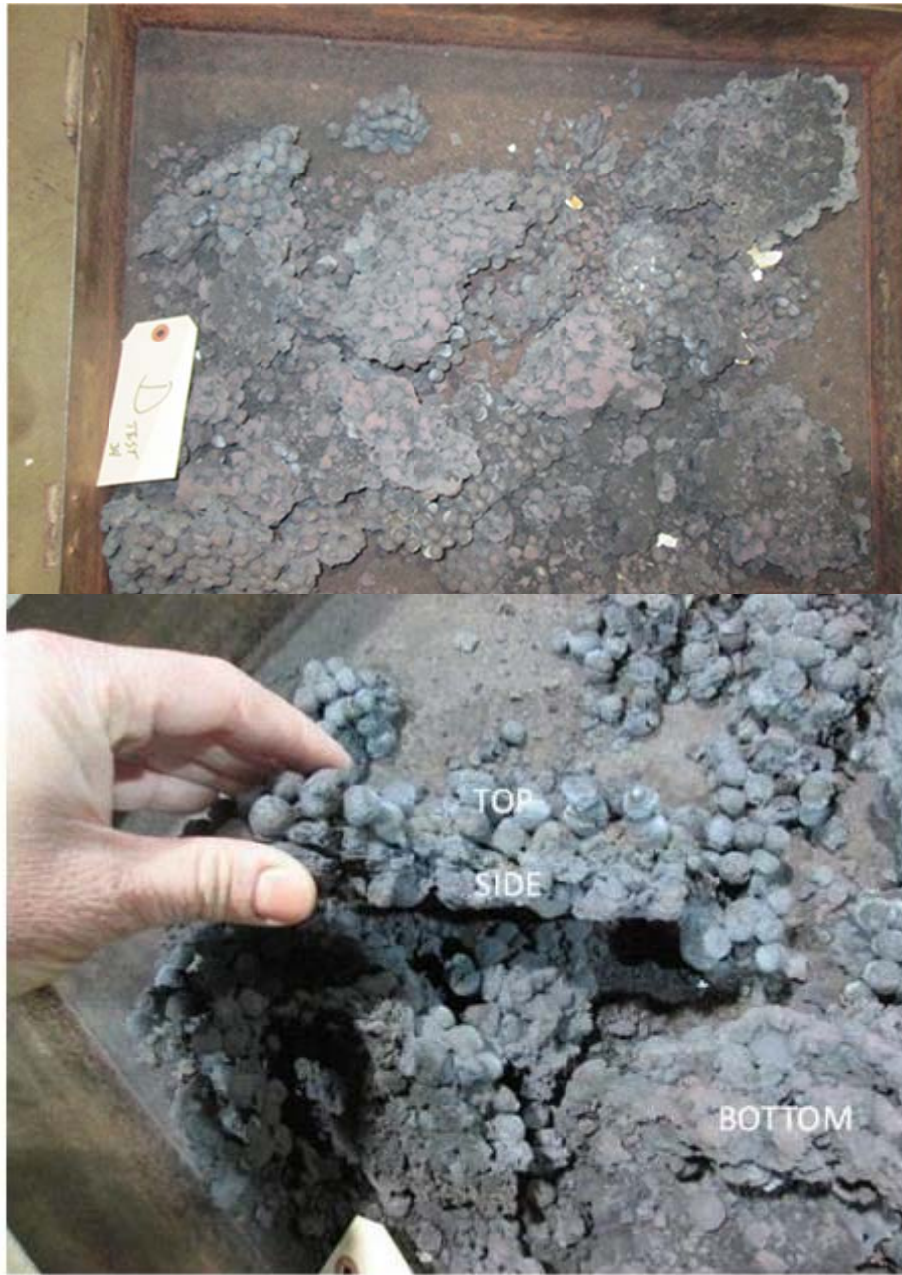
Figure 45. DRI produced at a furnace hot-zone temperature of 1400°C and residence time of 80 min. Dried greenballs which contain revert material (14-5) (molar C/O ratio = 1.1) were used as a feed material. The initial bed height of the dried greenballs was 7.6 cm. The DRI was cooled in the LHF cooler at a long residence time, and then was shoveled out to a tray and further cooled in nitrogen under the external hood.
