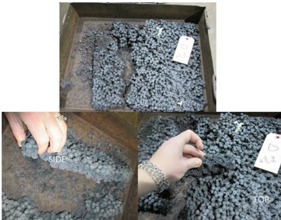
Figure 48. DRI produced at a furnace hot-zone temperature of 1450°C and residence time of 80 min. Dried greenballs which contain revert material (14-5) (molar C/O ratio = 1.1) were used as a feed material. The initial bed height of the dried greenballs was 7.6 cm. The DRI was cooled in the LHF cooler at a long residence time, and then was shoveled out to a tray and further cooled in nitrogen under the external hood.
