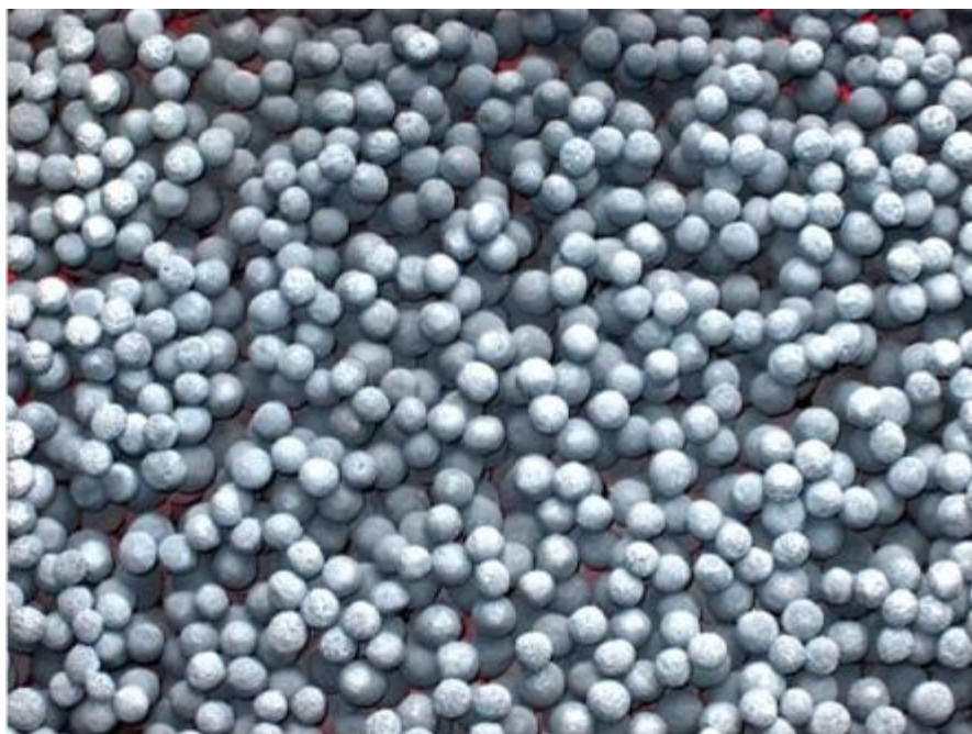
Figure 43. DRI located at the top layer in cart 6 from the experiment conducted to simulate continuous operation. Dried greenballs which contain magnetite concentrate (greenball recipe 13-2) (molar C/O ratio = 1.2) were used as a feed material. The initial bed height was 10.2 cm. The DRI was cooled in the LHF cooler at a long residence time.
