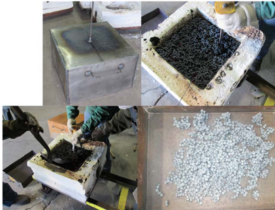
Figure 19. DRI produced using dried greenballs which contain magnetite concentrate (greenball recipe 14-6) (molar C/O ratio = 1.1) at an initial bed height of 7.6 cm, and furnace temperature of 1500°C, and residence time of 80 min. The DRI was cooled in the LHF cooler (long residence time) then shoveled out of the cart into a pan. The pan was placed under the cooling hood, and purged with nitrogen for complete cooling of the DRI.
