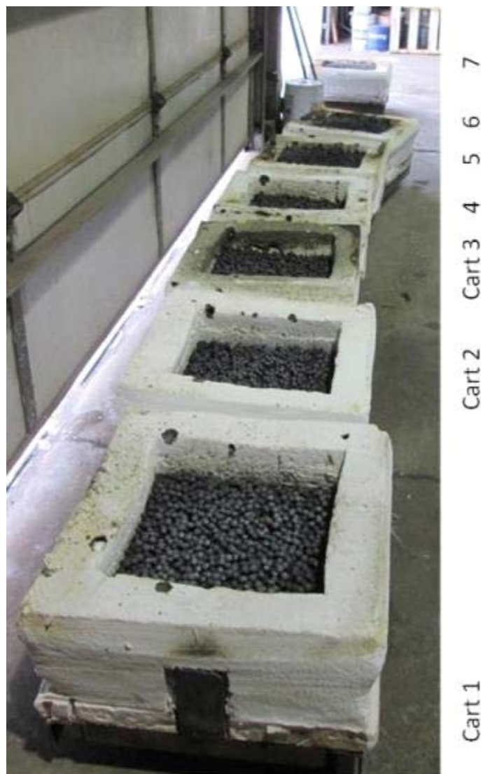
Figure 42. DRI produced in carts 1 through 7. Dried greenballs which contain magnetite concentrate (greenball recipe 13-2) (molar C/O ratio = 1.2) were used as a feed material. For carts 1 through 4, the initial bed height was 7.6 cm, and for carts 5, 6, and 7 the initial bed height was 10.2 cm. DRI produced was cooled in the LHF cooler at a long residence time.
