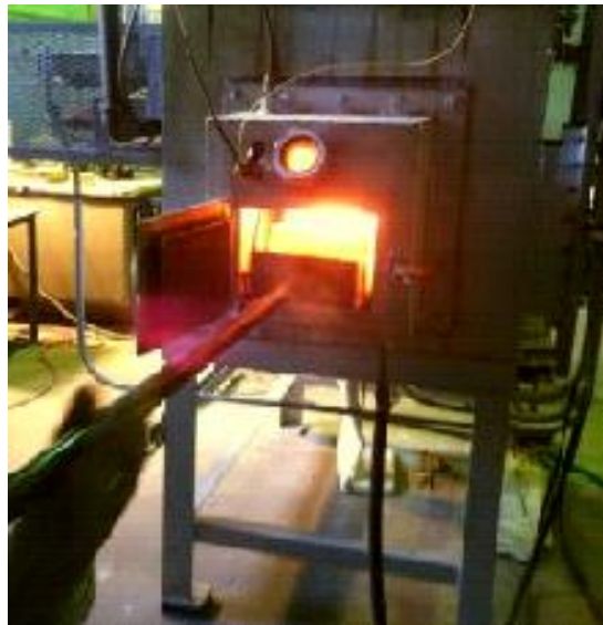
Figure 53: Moving Sample Tray through Furnace
