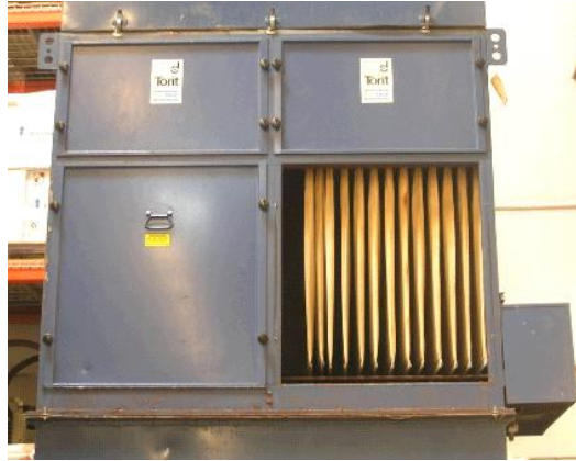
Figure 15. Bag house installed at Large Batch Furnace facility.
