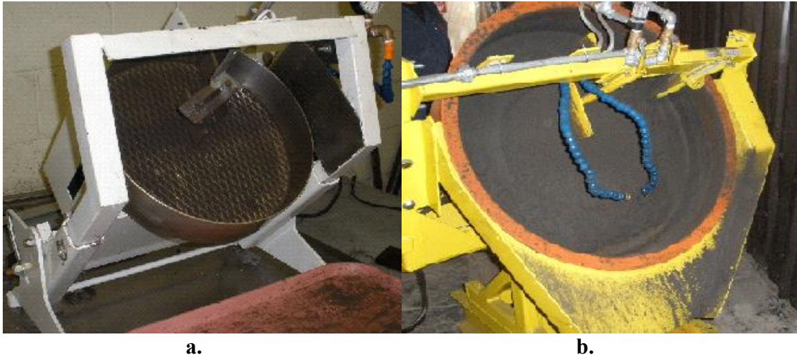
Figure 2. Pelletizing Discs at Mars Mineral (not to scale).
