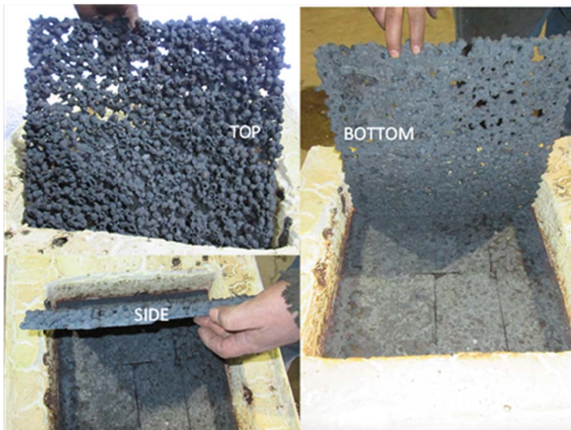
Figure 70 . DRI produced using dried greenballs which contain revert material (dried greenball recipe 14-8) (molar C/O ratio = 1.0) at a furnace temperature of 1500°C and residence time of 80 min. For the DRI shown, the initial bed height was 5.1 cm. The DRI was cooled in the LHF cooler at a long residence time.
