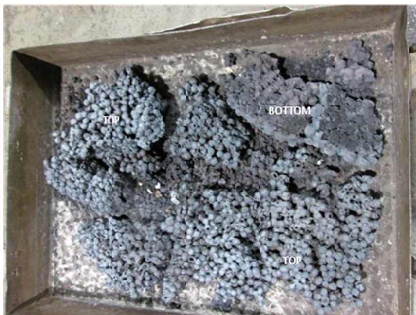
Figure 51. DRI produced at a furnace hot-zone temperature of 1500°C and residence time of 80 min. Dried greenballs which contain revert material (14-5) (molar C/O ratio = 1.1) were used as a feed material. The initial bed height of the dried greenballs was 7.6 cm. The DRI was cooled in the LHF cooler at a long residence time, and then was shoveled out to a tray and further cooled in nitrogen under the external hood.
