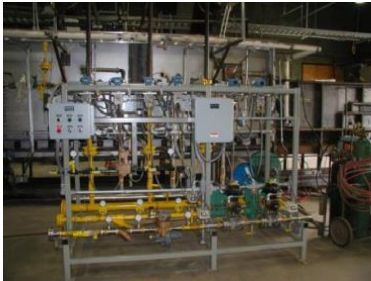
Figure 11. Oxygen – Fuel combustion system valve train.
