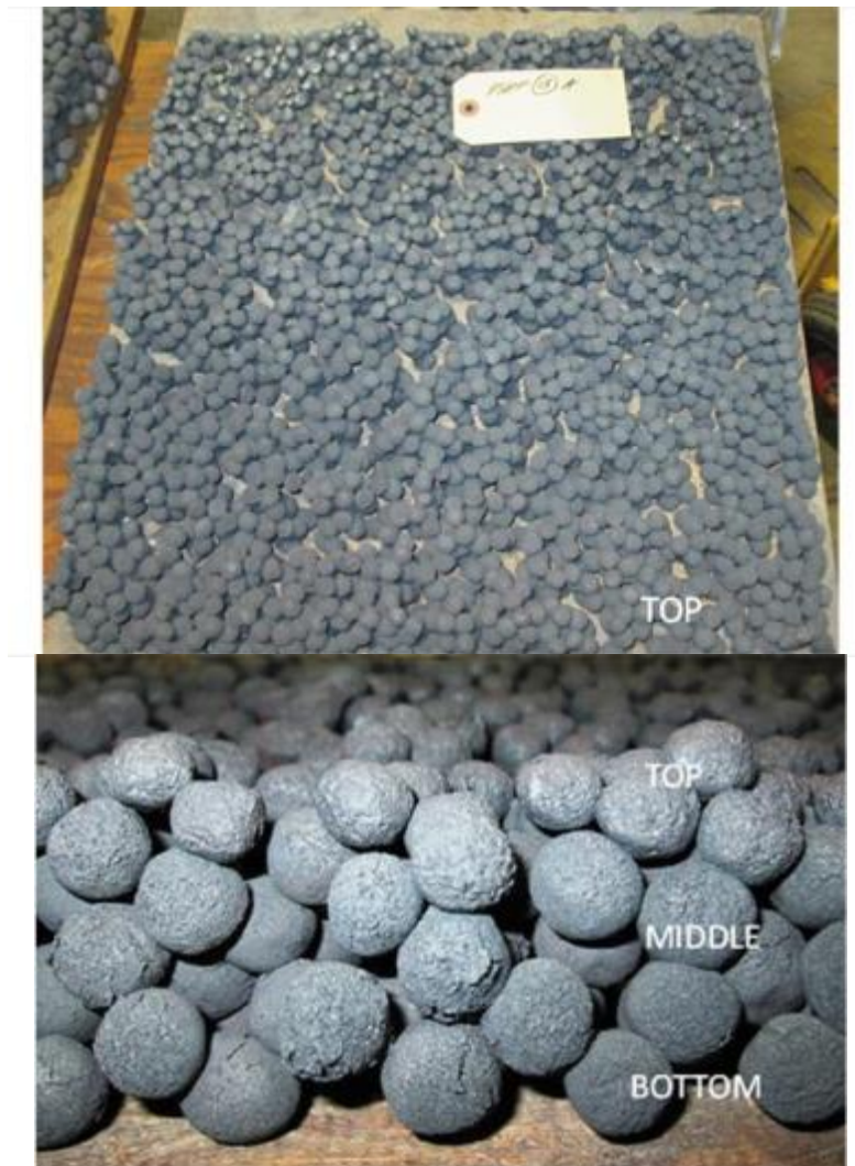
Figure 36. DRI produced at a furnace temperature of 1475°C, and residence time of 80 min using dried greenballs which contain magnetite concentrate (greenball recipe 13-1) (molar C/O ratio = 1.0) at an initial bed height of 7.6 cm. DRI produced throughout these experiments was cooled in the LHF cooler at a long residence time.
