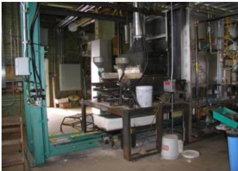
Figure 14. LHF moving cart system, feed end.
