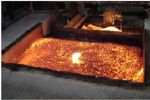
Figure 4. Appearance of reduced pellets after test in Large Batch Furnace, Version 1. (Note melted area on reduced pellet surface on lower left corner of pallet.)
