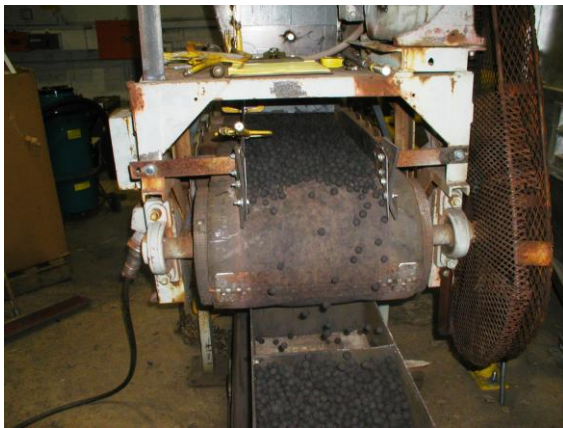
Figure 13. Green Ball Feeding Hearth Simulator (Initial Test)
