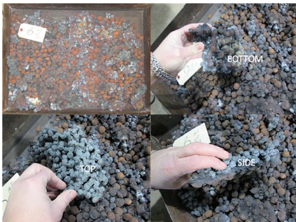
Figure 47. DRI produced at a furnace hot-zone temperature of 1450°C and residence time of 50 min. Dried greenballs which contain revert material (14-5) (molar C/O ratio = 1.1) were used as a feed material. The initial bed height of the dried greenballs was 7.6 cm. The DRI was cooled in the LHF cooler at a long residence time, and then was shoveled out to a tray and further cooled in nitrogen under the external hood.
