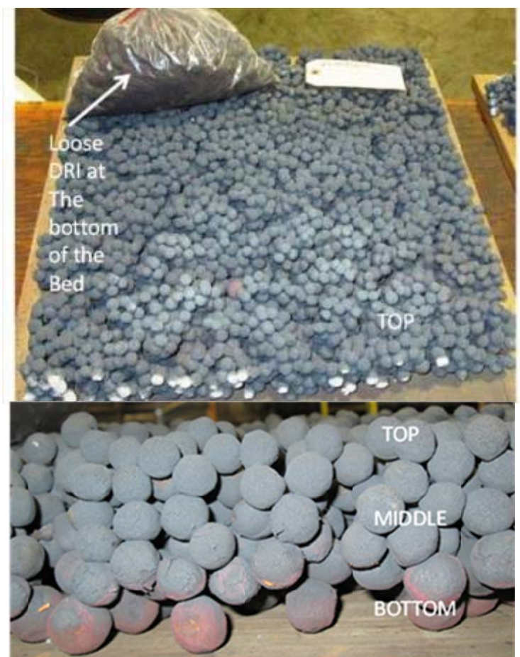
Figure 38. DRI produced at a furnace temperature of 1475°C and residence time of 80 min using dried greenballs which contain magnetite concentrate (greenball recipe 13-1) (molar C/O ratio = 1.0) at an initial bed height of 12.7 cm. DRI produced throughout these experiments was cooled in the LHF cooler at a long residence time.
