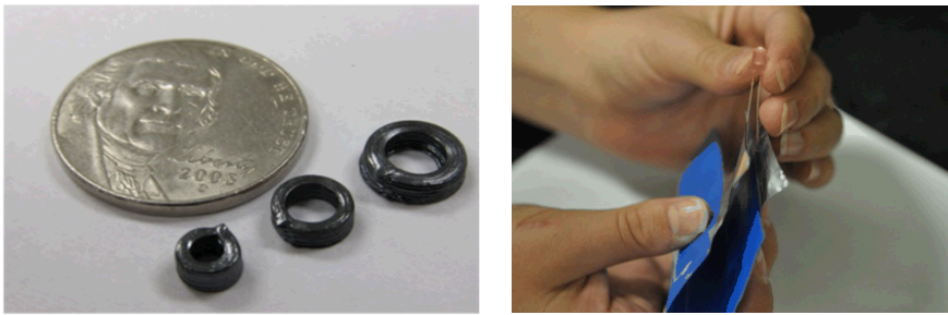
Printed power system components including ferrite based transformers and \text{LiFePO}_4 flexible batteries
