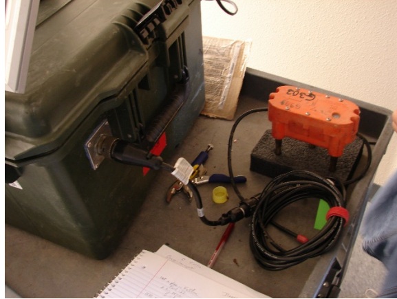
Figure A3 shows an L28 sensor ( https://www.passcal.nmt.edu/webfm_send/1186 ) which works with a RT130 digitizer ( https://www.passcal.nmt.edu/content/instrumentation/dataloggers/3-channel-dataloggers/reftek-rt-130-datalogger ). The sensor dimensions are 8x20x6 cm with 8 cm spikes. The sensor is stored in a BIHO box as in Figure A4.
