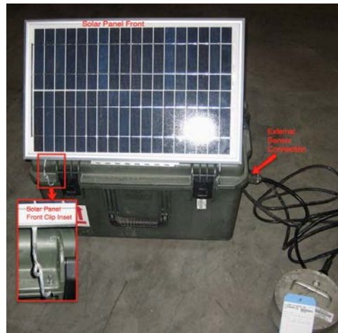
Figure A6 shows the BIHO box solar panel and a short-period sensor larger than the one we would use.
