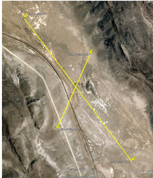
Figure 1. Three days of ambient noise were recorded by a deployment of ~350 high-frequency geophones equipped with "Texan" digitizers co-located with an active source survey. The inter-sensor distance was 15 m. Line 4 is parallel to the road, line 6 is perpendicular to the road.
