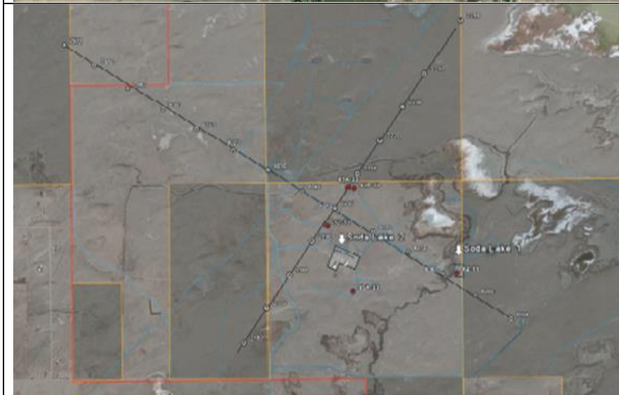
Figure 1B shows the 2010 active source test lines (black) as reported by Echols, (2011). Our ambient seismic noise deployment was at the same location as the Line 2 (black line trending northwest-southeast). This location was suggested by Mr. James Echols (formerly of Magma), as a location where faults were interpreted and where the active survey had inconclusive S-arrival results, specifically near the power plant (southeast portion of Line 2 (James Echols, personal communication)).
