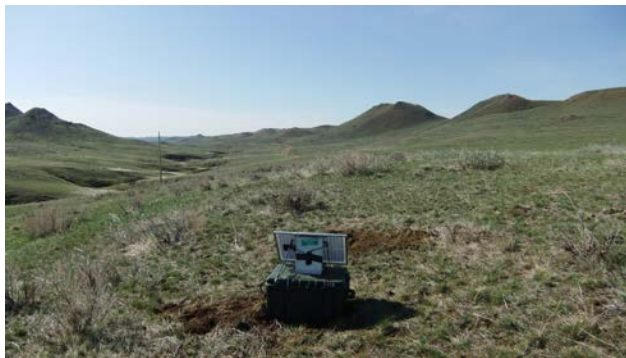
Figure A3 shows an L28 sensor ( https://www.passcal.nmt.edu/webfm_send/1186 ) which works with a RT130 digitizer ( https://www.passcal.nmt.edu/content/instrumentation/dataloggers/3-channel-dataloggers/reftek-rt-130-datalogger ). The sensor dimensions are 8x20x6 cm with 8 cm spikes. The sensor is stored in a BIHO box as in Figure A4.
