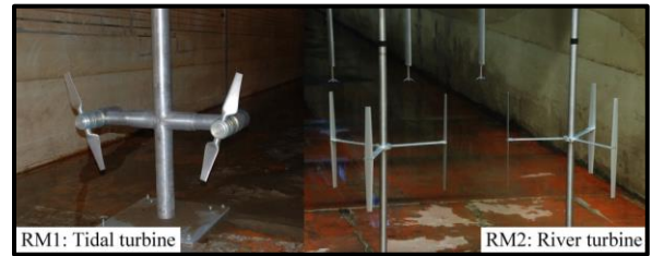
FIG. 1: 1:40 SCALE AXIAL-FLOW RM1 AND 1:15 SCALE CROSS-FLOW VERTICAL AXIS RM2 TURBINES INSTALLED AT THE UMN-SAFL FACILITY.
