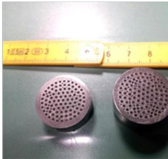
Figure 6.1.47. Restacking of the 91 monocoil wires into the Monel outer sheath
