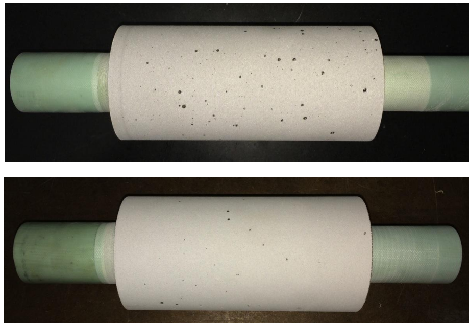
Figure 6.3.5. Top: First attempt of support cylinder manufacturing with numerous voids on the outer machined surface. Bottom: Second improved cylinder with a significantly reduced number of voids
