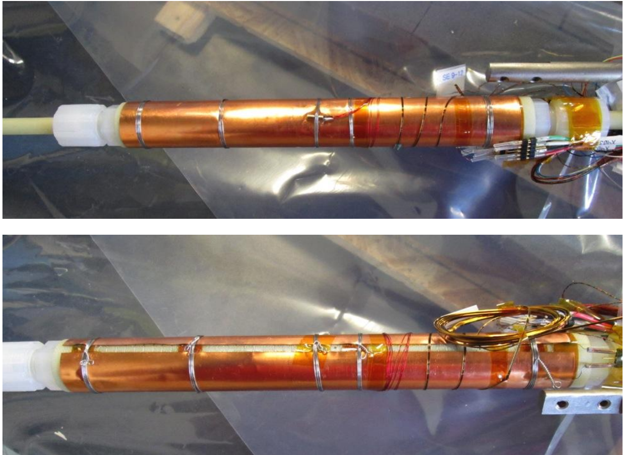
Figure 6.5.62. Calibration Heater Modification. A thin copper sheet was wrapped around the heater wire to ensure a uniform heater surface temperature. A Cernox™ temperature sensor was mounted on the copper surface to measure the heater surface temperature.
