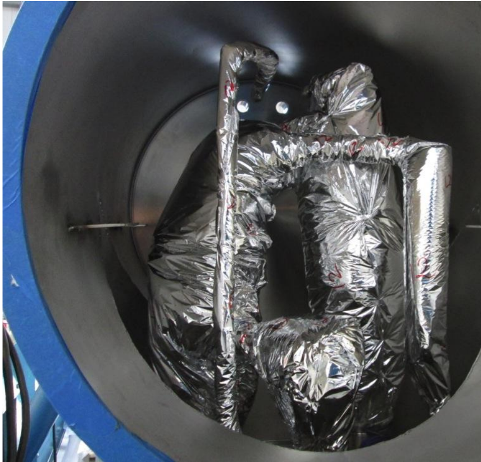
Figure 6.5.61. Cooling Module Insulation. All components inside the cooling module vacuum space are wrapped with 12 layers of multilayer insulation (MLI).
