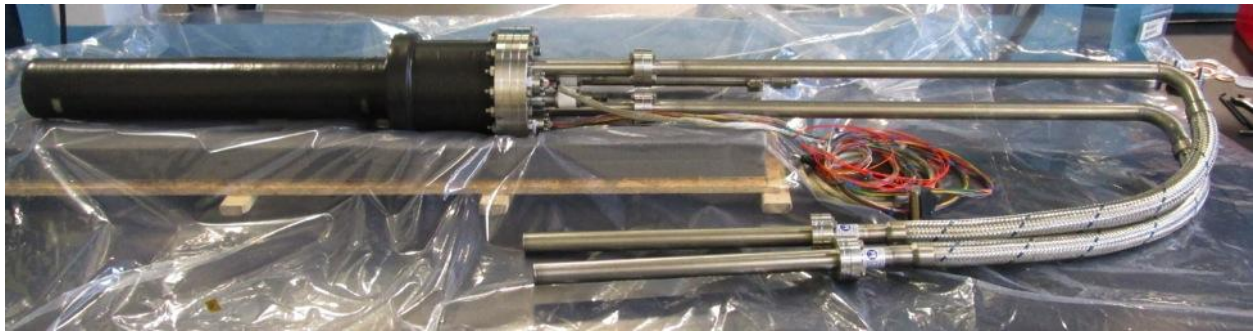
Figure 6.5.63. Cryogenic Transfer Line. The transfer line is shown installed on the experiment module.
