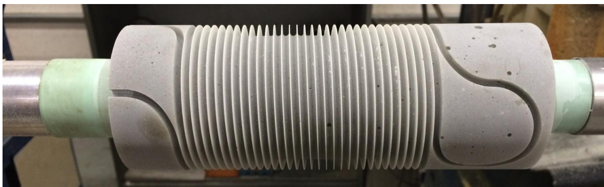
Figure 6.3.6. Support groove for the bifilar solenoidal winding machined into the support cylinder
