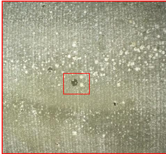
Figure 6.3.11. Enlarged view of the square shown in Figure 6.3.10, which contains a small void in the surface.
