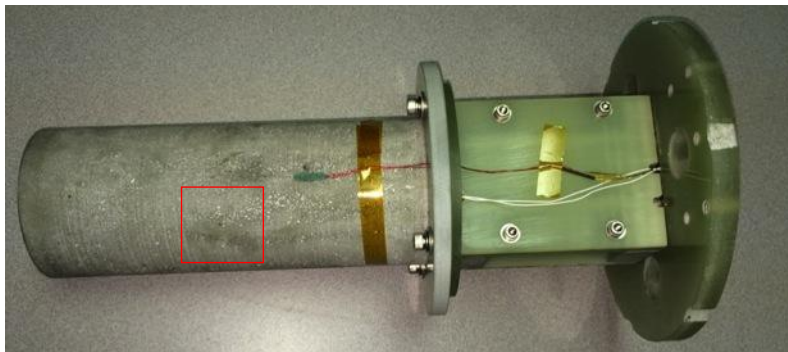
Figure 6.3.10. Test coil returned from fatigue test. The red square indicates an area of detailed surface inspection.
