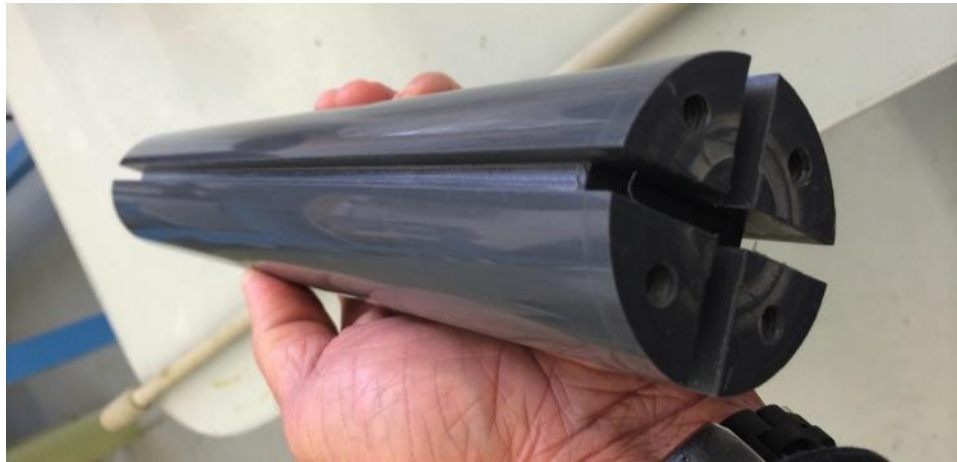
Figure 6.5.66. Support structure for pick-up coil for measurements of rotating magnetic field
