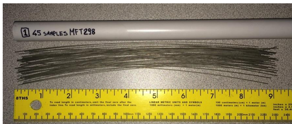
Figure 6.5.88. Straight MgB 2 wire samples used for magnetization loss measurements
