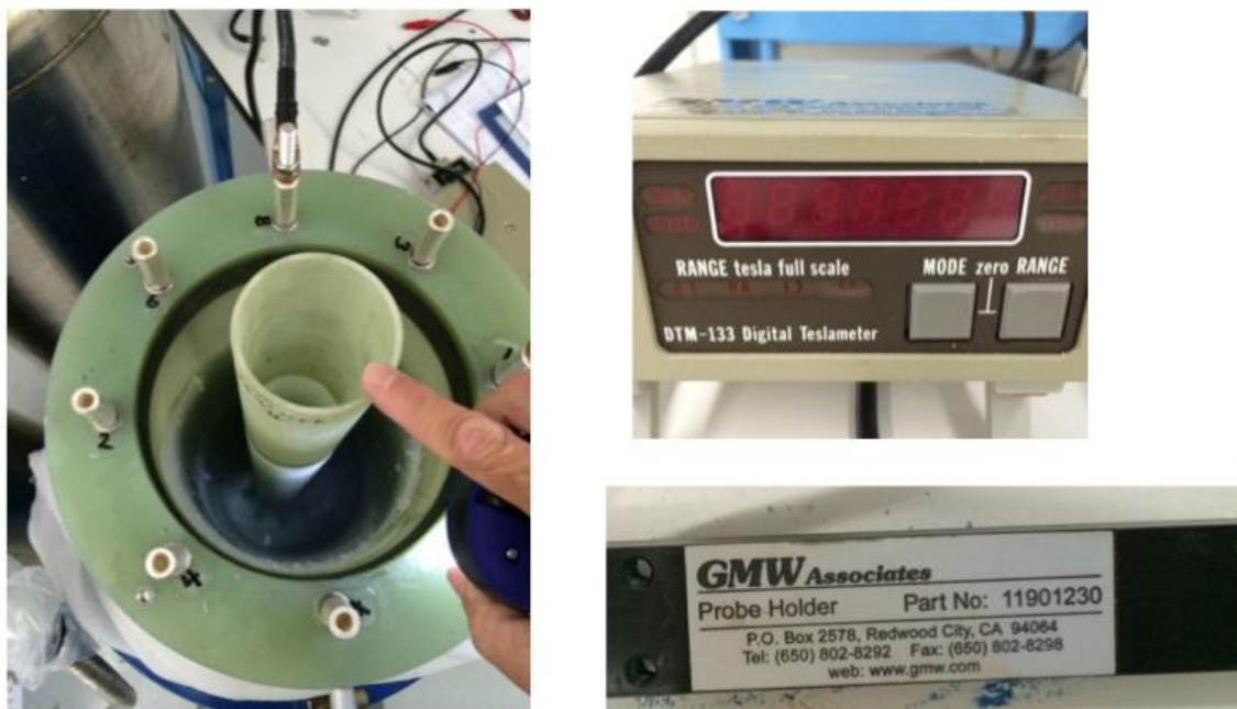
Figure 2 A GMW Associates Hall probe is used to measure the magnetic field. A warm bore was inserted into the coil assembly for the hall probe.
