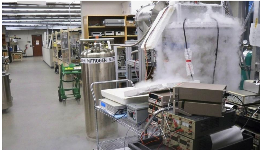
Figure 6.5.74. Operation of AC loss measurement system with LN2 boil-off
