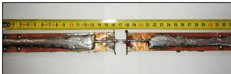
Figure 6.1.35. Mini cable prepared in the sample holder for I_c measurements
