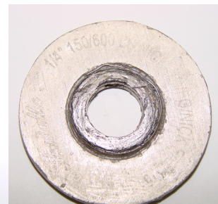
Figure 7c. Flexitallic gasket after cleaning.
