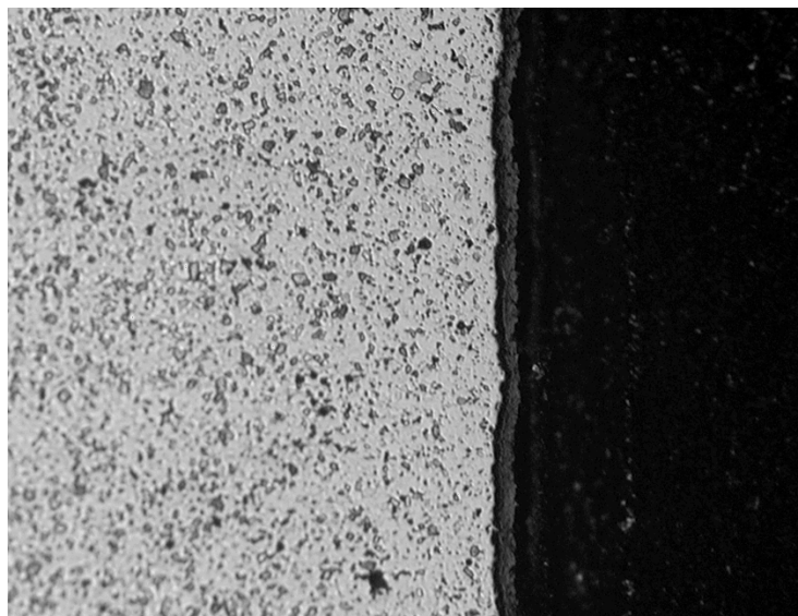
10-0108-56 Specimen #2 200X 20µm Murakami's Reagent SiC / outside end DIC
