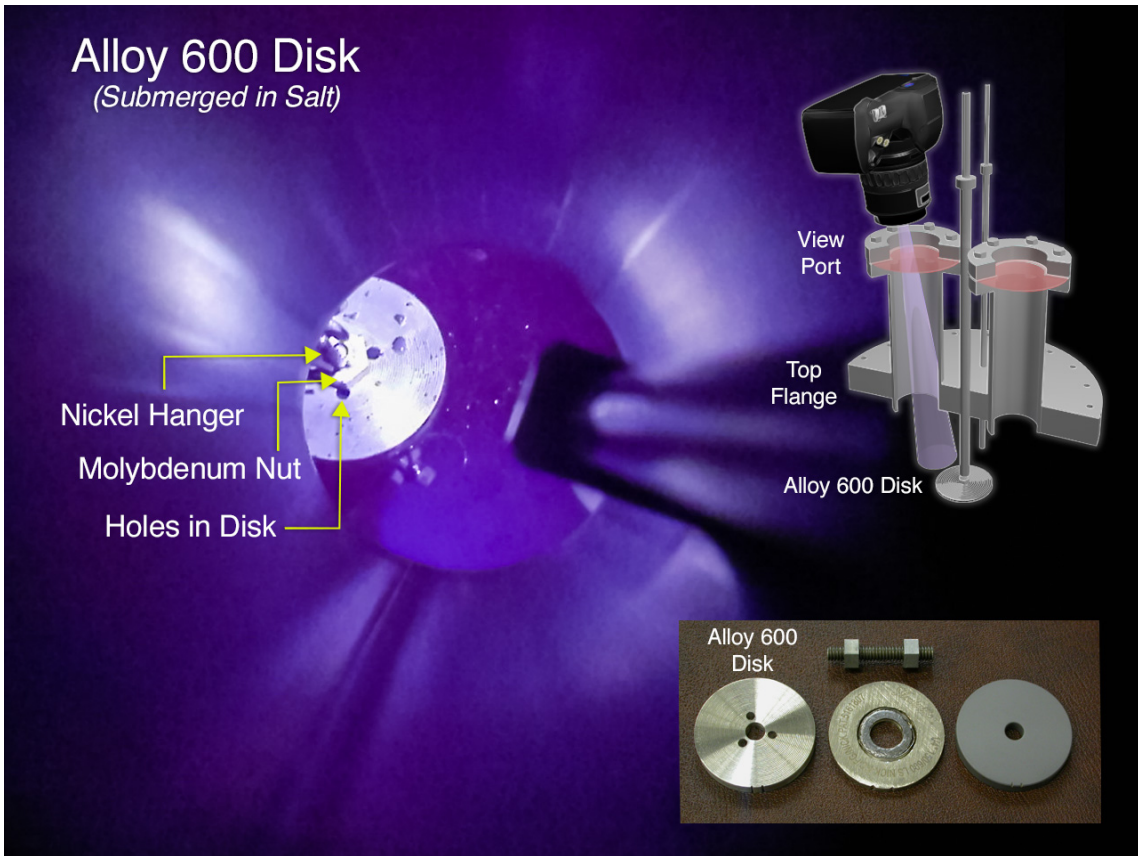
Figure 19. Specimen submerged in 700°C salt viewed through window.
