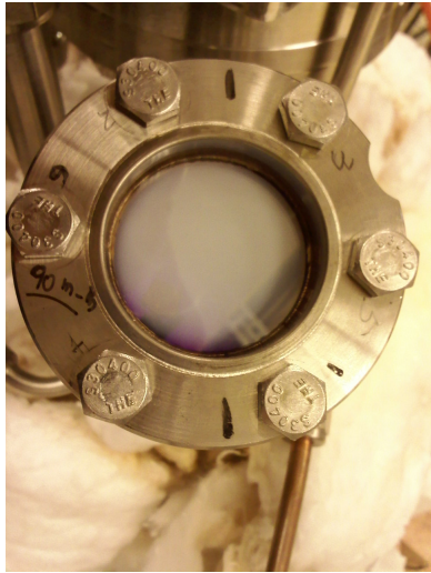
Figure 20. Sapphire window after one day at 700°C.
