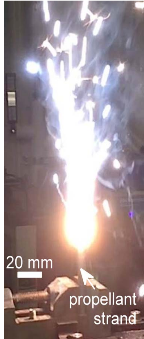
Figure 3: Digital photograph of aluminized propellant strand burner flame.
