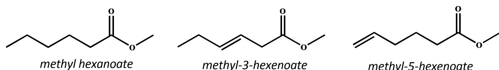
This experiment focuses on how the position of a double bond in the three compounds above affects HO<sub>2</sub> formation between 600 and 750 K. We selected these compounds because they **mimic the methyl ester portion of a biodiesel molecule**.
