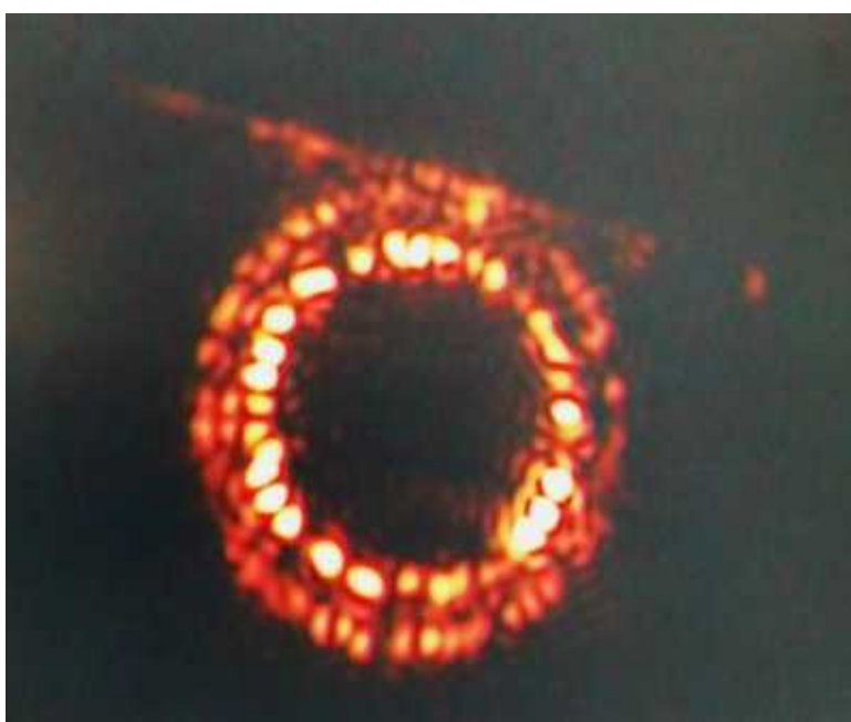
Second harmonic generation from LiNbO 3 disk
