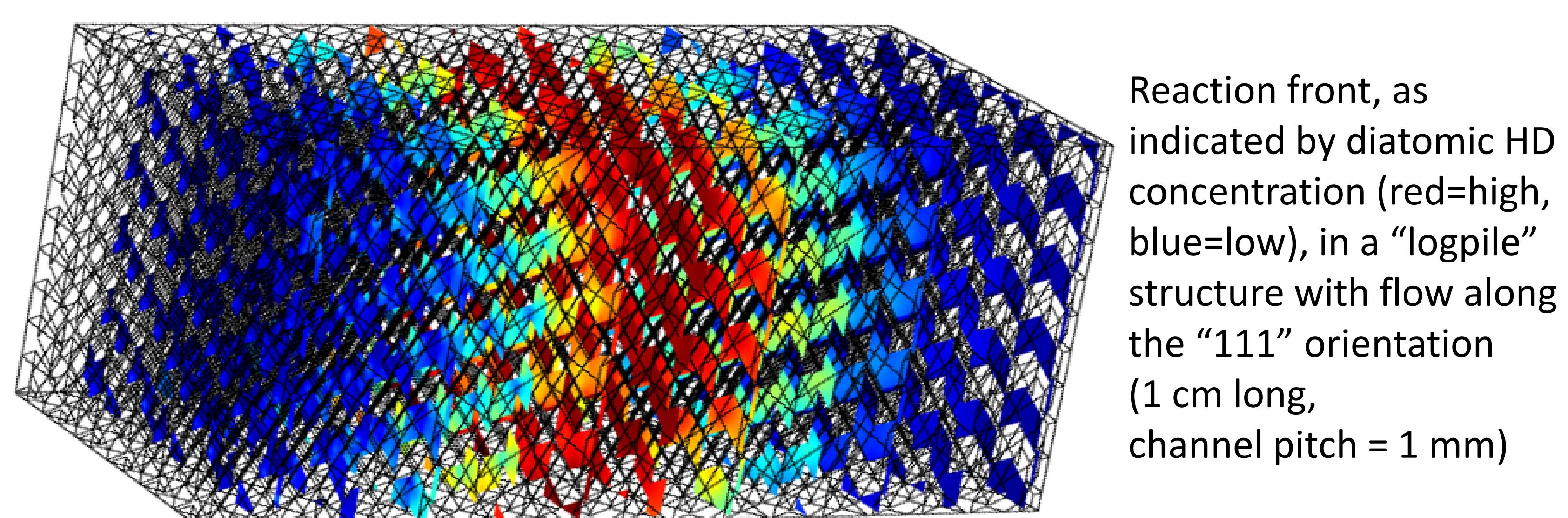
Reaction front, as indicated by diatomic HD concentration (red=high, blue=low), in a "logpile" structure with flow along the "111" orientation (1 cm long, channel pitch = 1 mm)
