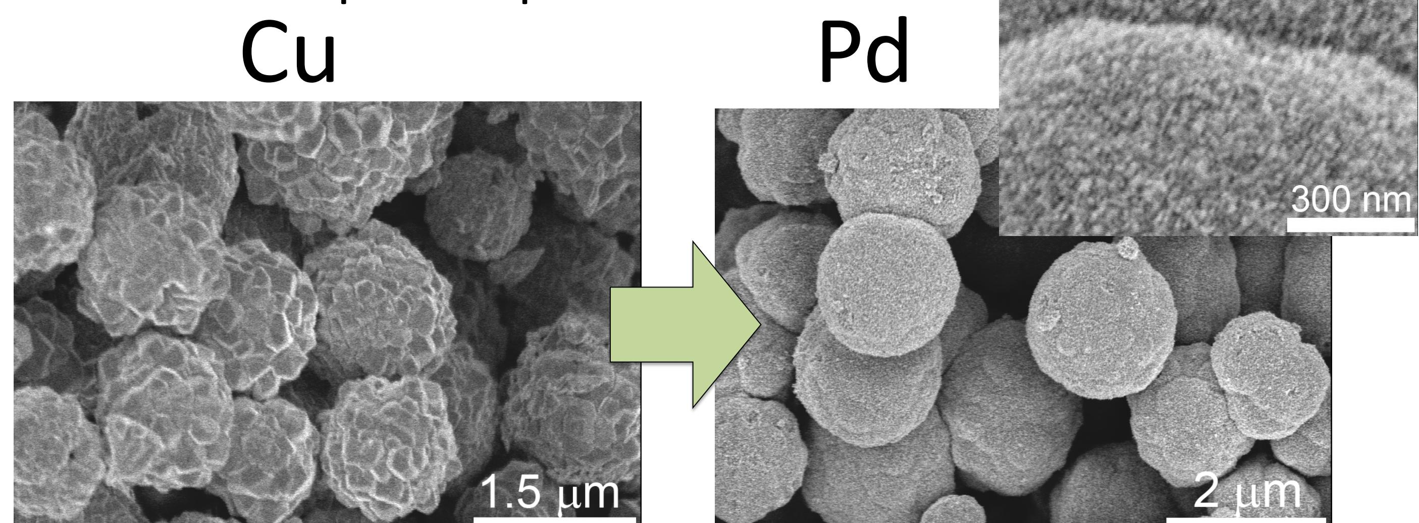
The reaction is geometrically self-limiting, preventing uncontrolled growth of the reduced metal particles.
