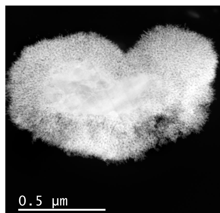
Nanoporous Pd can be grown on nonporous Pd particles to increase surface area for chemical reactions at the surface.
