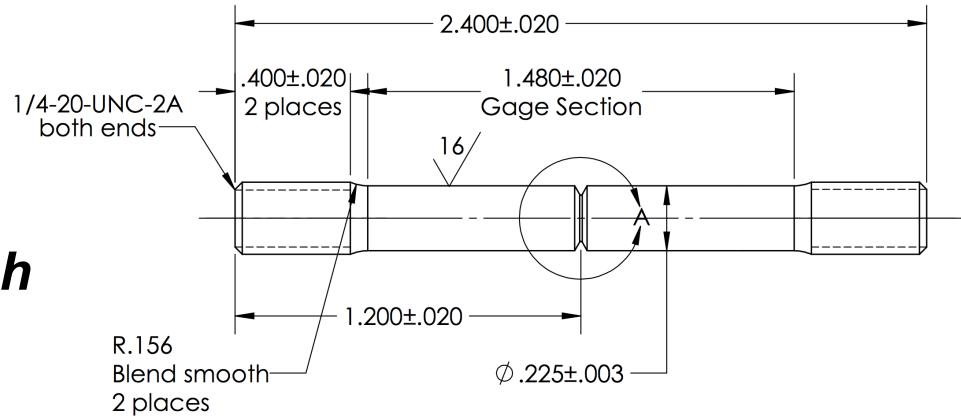
$$K_{t, \text{elastic}} \sim 3.9 \quad K_{t, \text{elastic-plastic}} \sim 2.4$$
