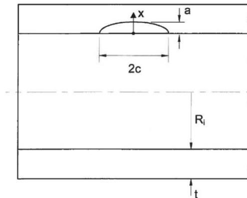
Semi-elliptical defect size and shape:
