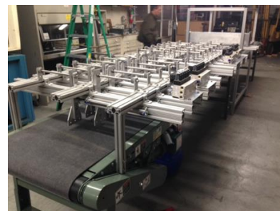
Figure 2. (top) 30 kV, 36" wide X-ray source. (bottom) The UHV pilot scale aluminum alloy sorting system
