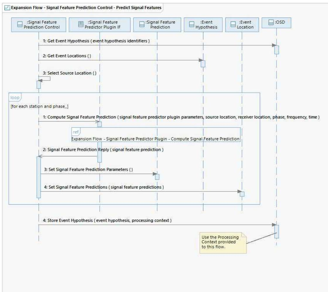
This flow shows Signal Feature Prediction Control predicting signal features using the Signal Feature Predictor Plugin IF. Signal Feature Predictor Plugin IF implementations may predict different types of signal features such as travel time, azimuth, slowness, amplitude, and probability of detection.
