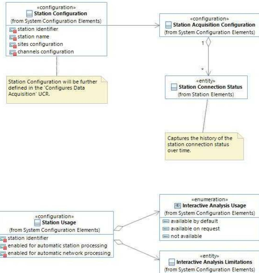
This diagram shows the Station Configuration class and related classes describing the Station's connections to the System and operational usage.
