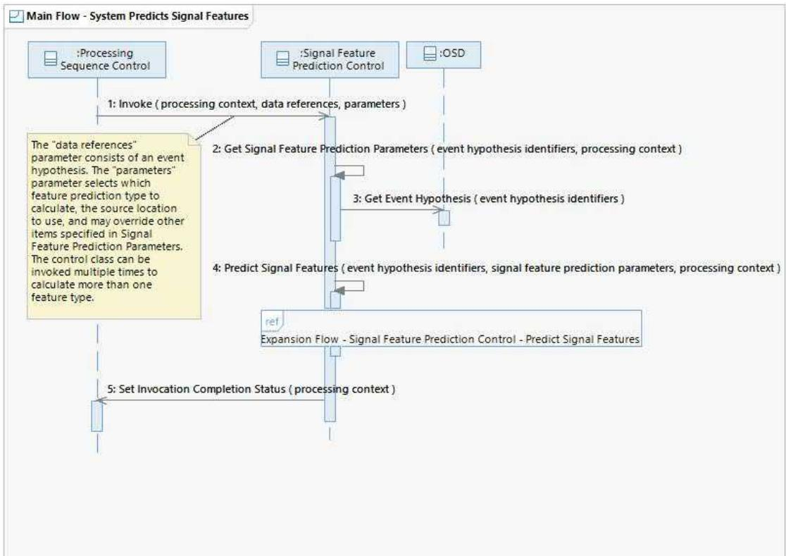
This flow shows how the system predicts signal features. The flow is stimulated by the Processing Sequence Control mechanism as part of executing an automatic processing sequence. The precise triggering conditions for such sequences are configured by the System Maintainer (see "Defines Processing Sequence" UCR). For more information about the Processing Sequence Control mechanism see "System Detects Event" UCR.
