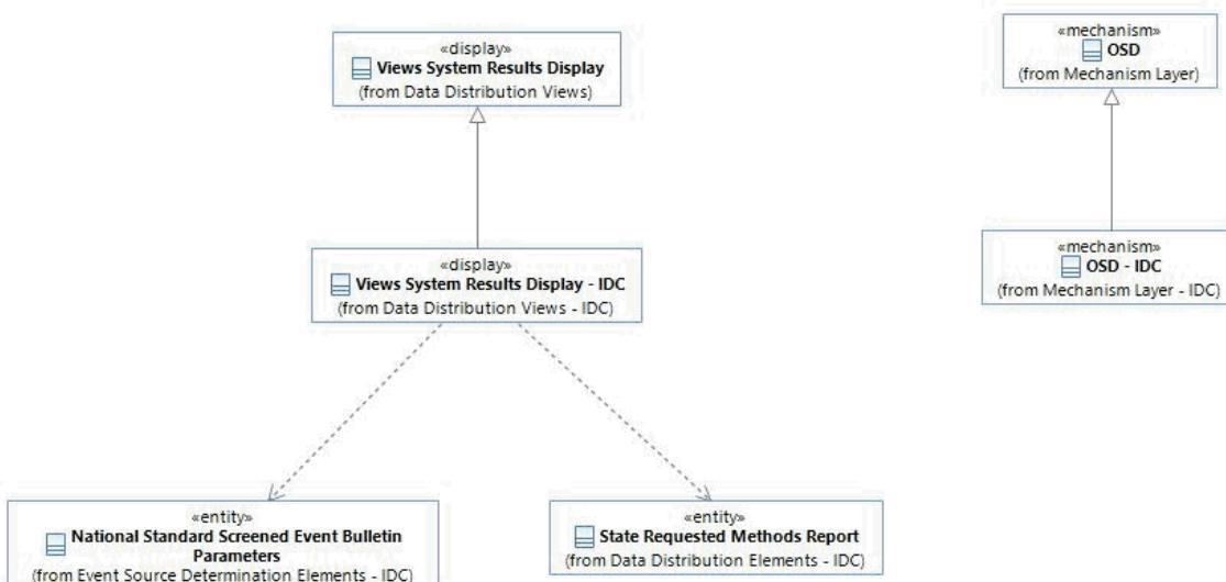
This diagram shows IDC specific classes related to providing System results to the Authorized External User via the Views System Results Display. The IDC specific Views System Results Display provides the Authorized External User the capability to search for and view Automated Warning/Notification Parameters and IDC only products such as the State Requested Methods
