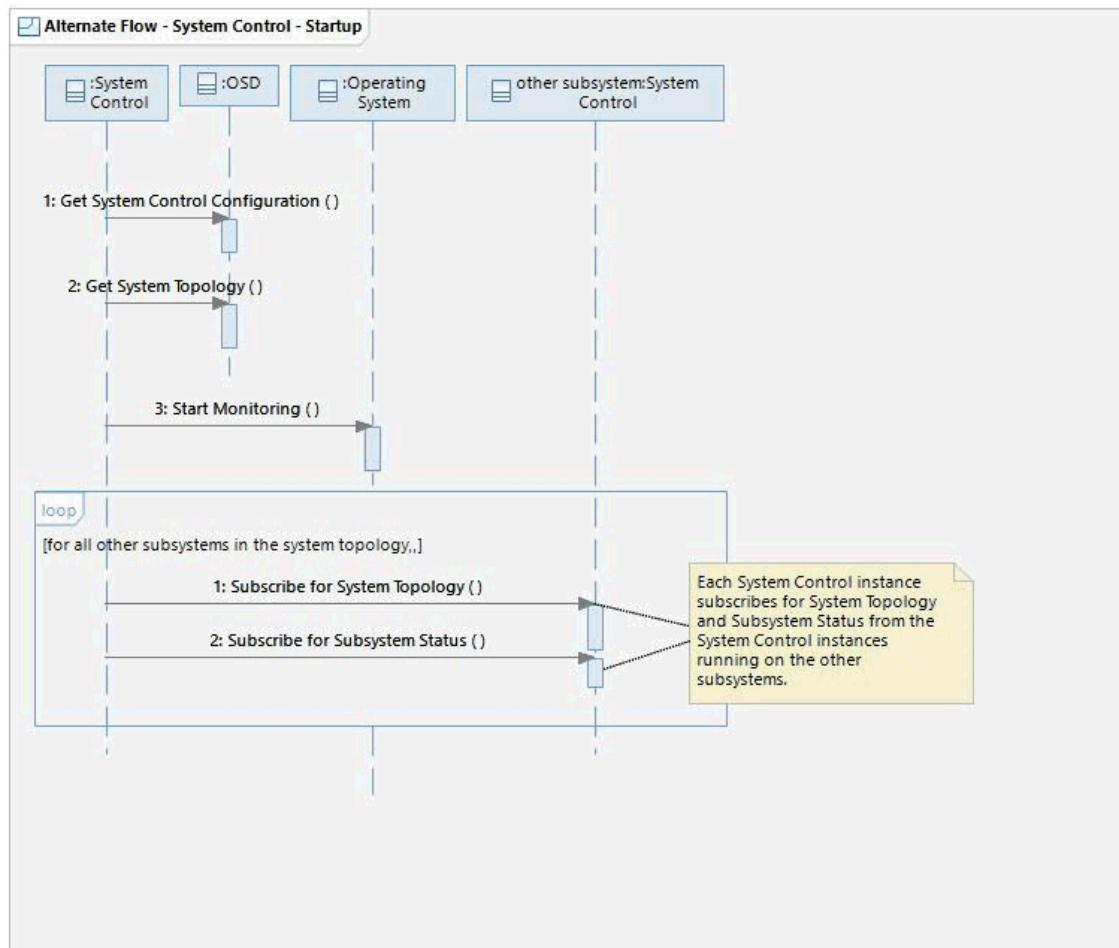
This flow shows actions performed by System Control when it first starts up. Each System Control instance in the topology subscribes for Subsystem Status and System Topology from the other instances.
