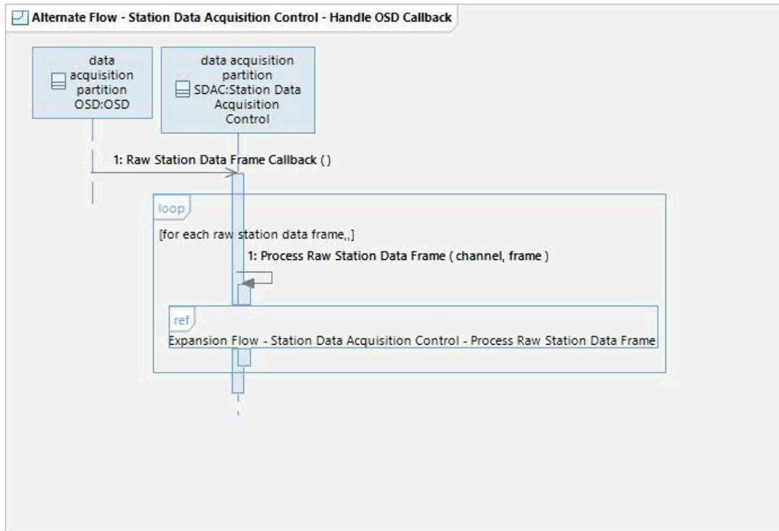
This flow depicts how the Station Data Acquisition Control handles a callback from the OSD to process raw station data frames that have been stored.
