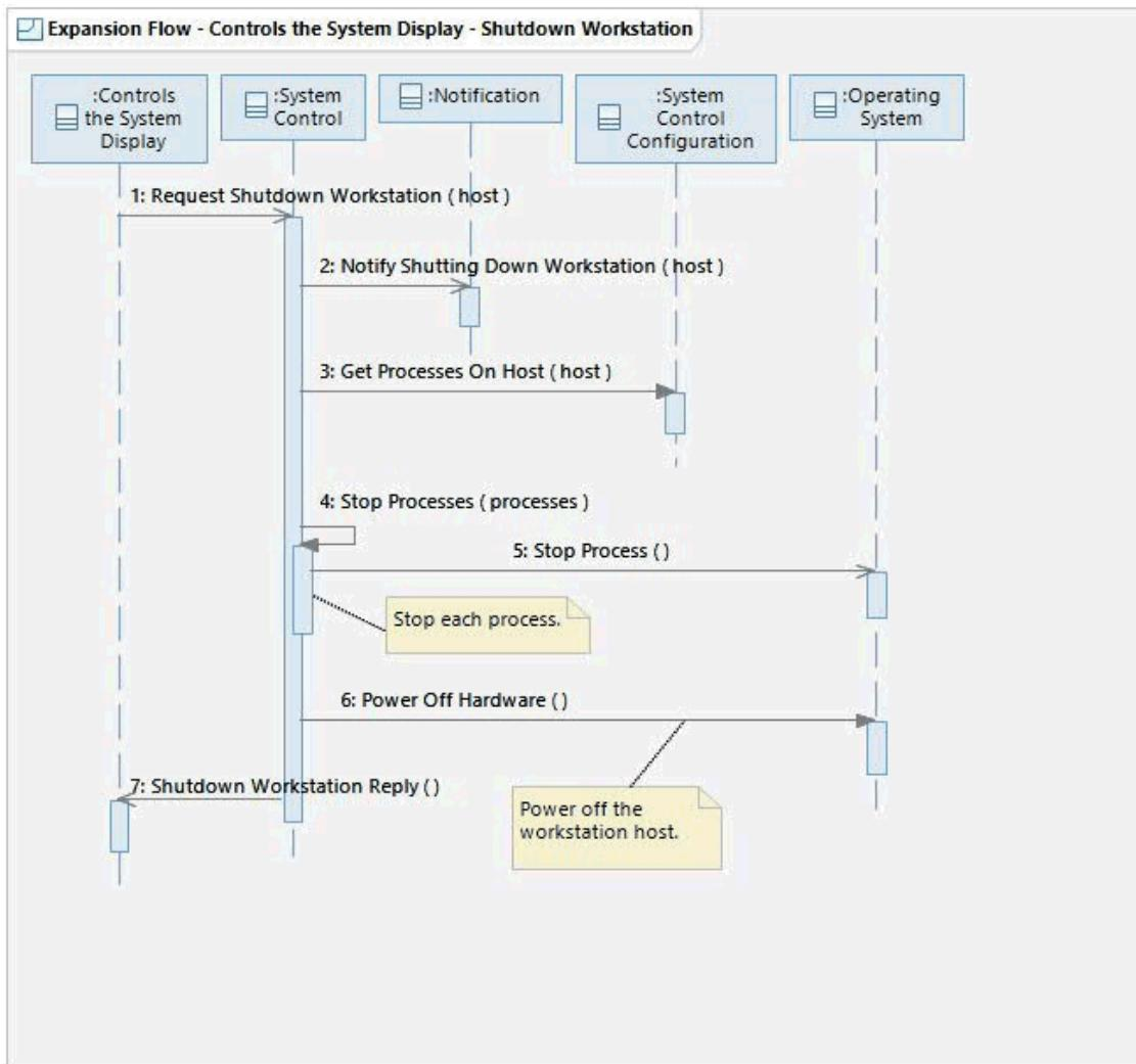
This flow shows how the Controls the System Display shuts down a workstation. This flow receives the workstation shutdown, which the System Controller selected in the invoking flow. System Control stops all the processes on the workstation and powers it off.
