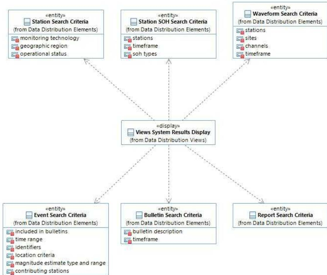
This diagram shows the various search criteria classes and details of those classes selected by the Authorized External User on the Views System Results Display. Though not shown on this diagram, the display class provides the criteria to the External System Results Control class which searches the OSD for classes matching the criteria, filters them based on user permissions, and returns them to the display for presentation to the Authorized External User.
