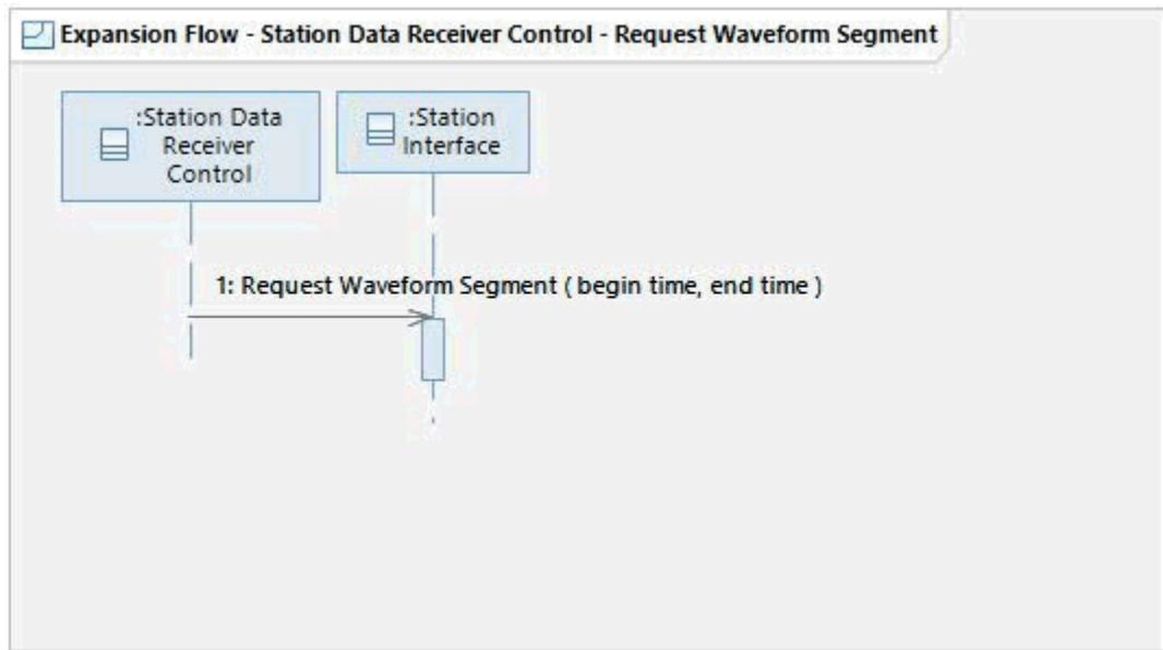
This flow shows Station Data Receiver Control requesting a waveform segment from a station. The station asynchronously provides the requested segment to Station Data Receiver Control (see “Main Flow – System Receives Station Data”).
