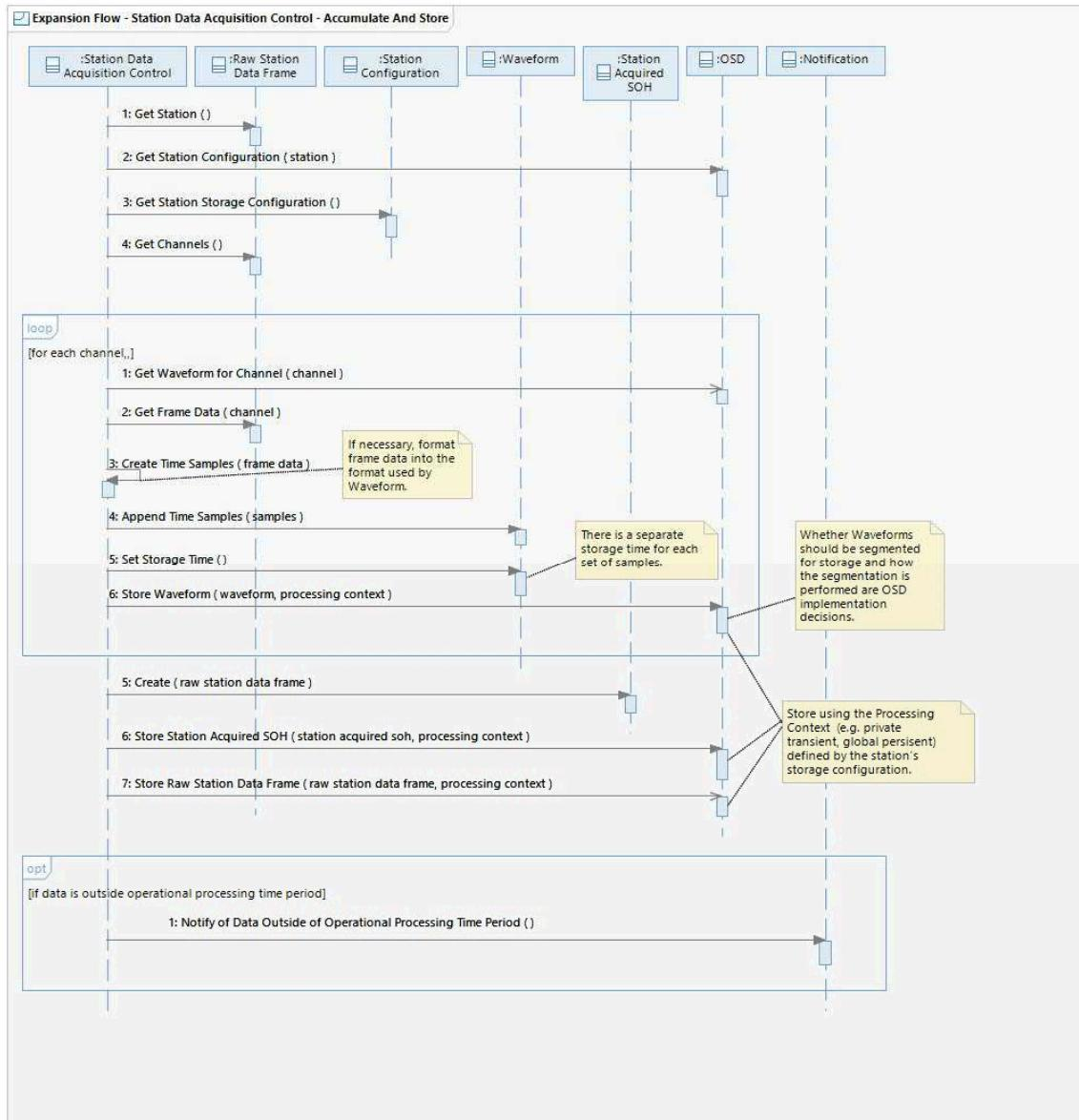
This flow describes how the Station Data Acquisition Control accumulates Raw Station Data Frames into Waveforms. Station Data Acquisition Control accumulates Raw Station Data Frames in Waveform objects (one Waveform for each channel in the Raw Station Data Frame) and stores the Waveforms in the OSD for use in automatic and interactive processing. Station Data Acquisition Control also parses Station SOH from the Raw Station Data Frame and stores the Station SOH object in the OSD.
