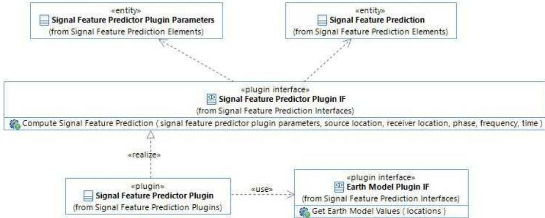
This diagram shows the Signal Feature Predictor Plugin IF, which is a common interface to all Signal Feature Predictor plugins. A Signal Feature Predictor Plugin may access plugins implementing the Earth Model Plugin IF.
