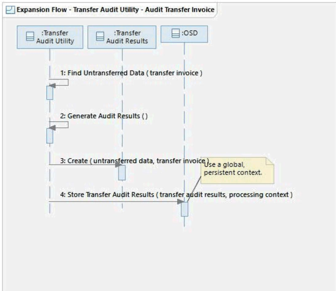
This flow is performed only on the receiving Data Acquisition Partition. The Transfer Audit Utility checks the OSD to determine if the data listed in the Transfer Invoice (e.g. Raw Station Data Frames, System Format Meteorological Data, bulletins, etc.) exists in the OSD, and creates and stores the Transfer Audit Results in the OSD.
