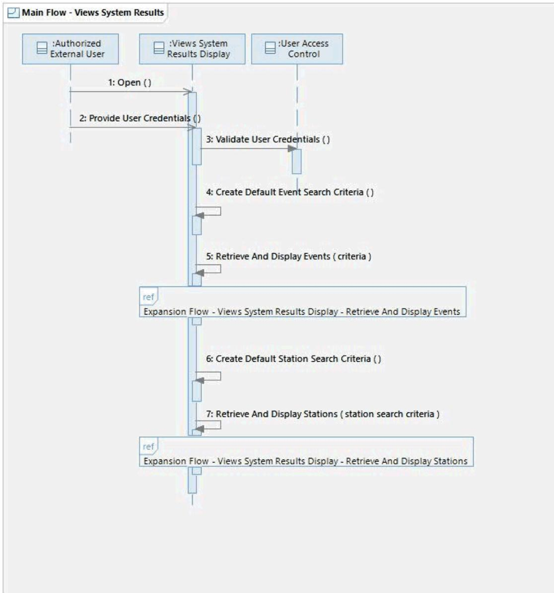
The flow shows the Authorized External User opening the Views System Results Display. The display uses the User Access Control mechanism to validate the user's credentials. The display performs default queries for Events and Stations and displays the results.
