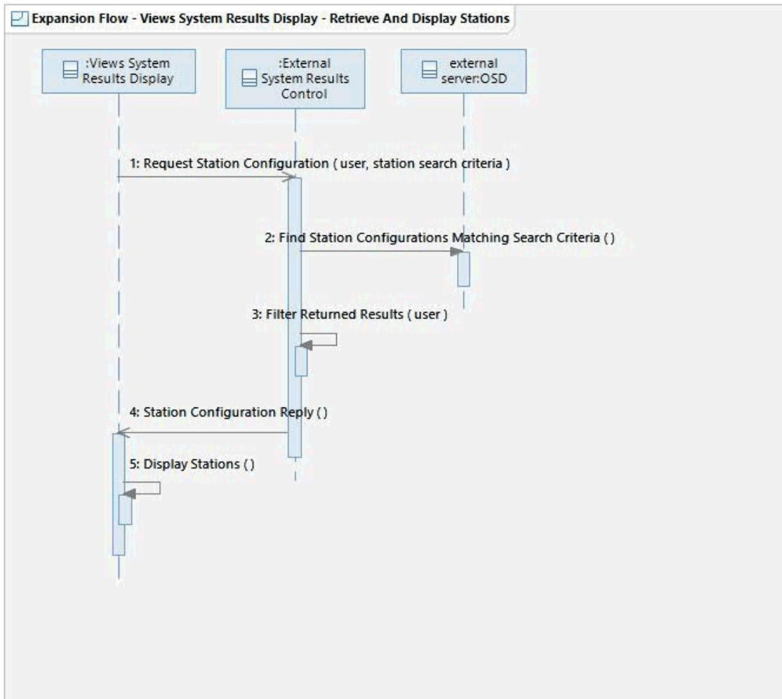
This flow shows how the Views System Results Display uses the External System Results Control to request Station configuration (location, instrumentation, site information, channel information, etc.) for display to the Authorized External User.
