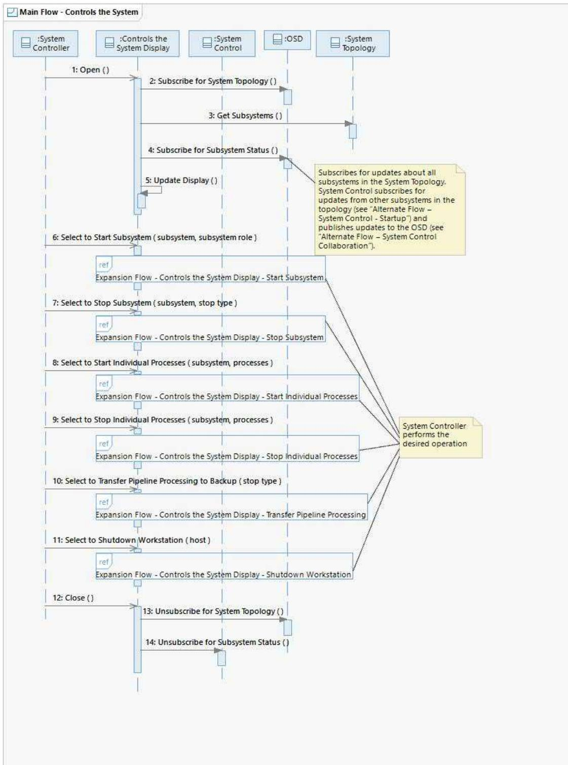
This diagram depicts the main flow. The System Controller controls the system via the "Controls the System Display". The display provides the ability to view the status of and control all subsystems in the System Topology.
