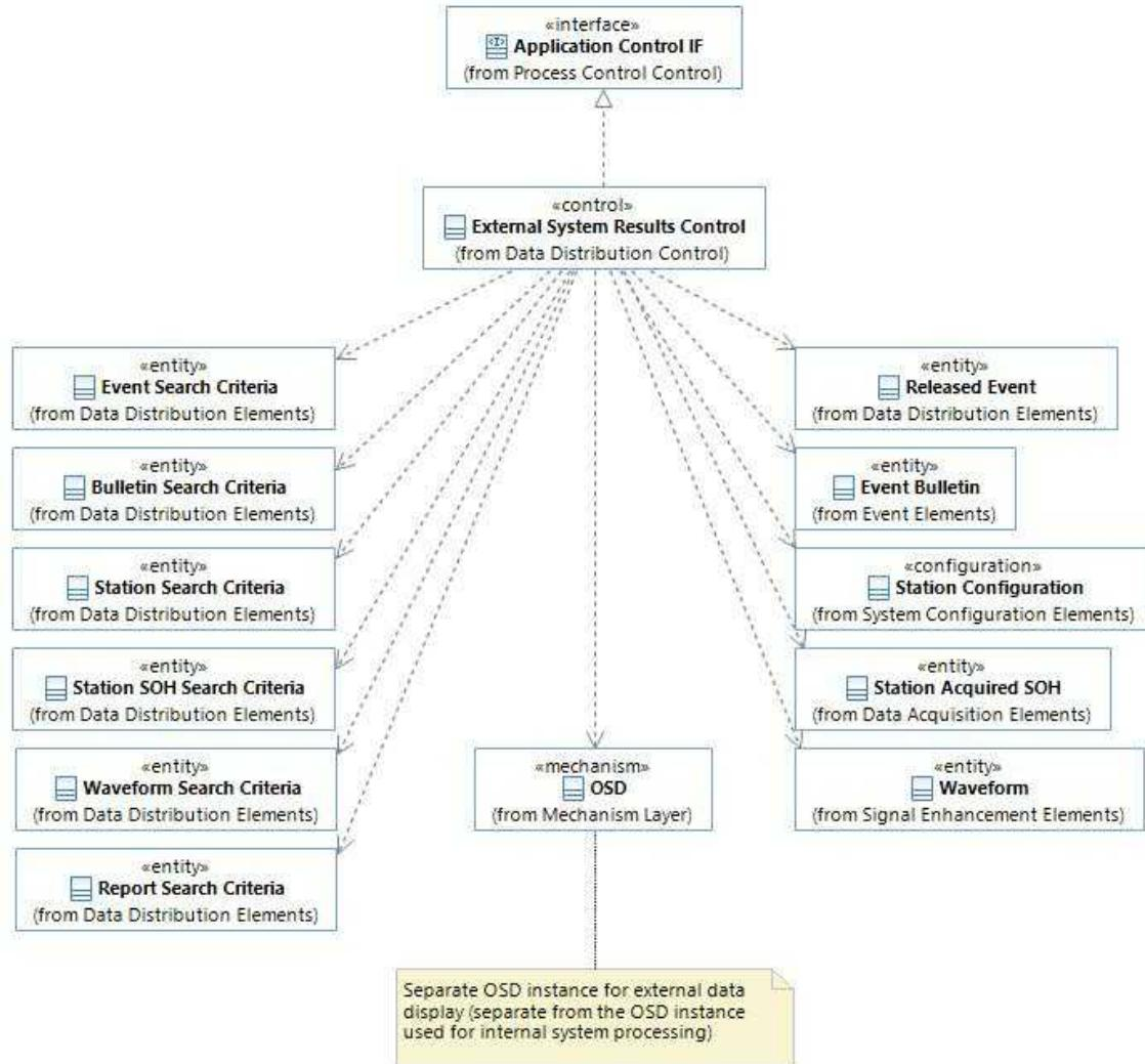
This diagram shows the External System Results Control class and related classes. The control class queries the OSD for in response to requests and search criteria provided by the Views System Results Display.
