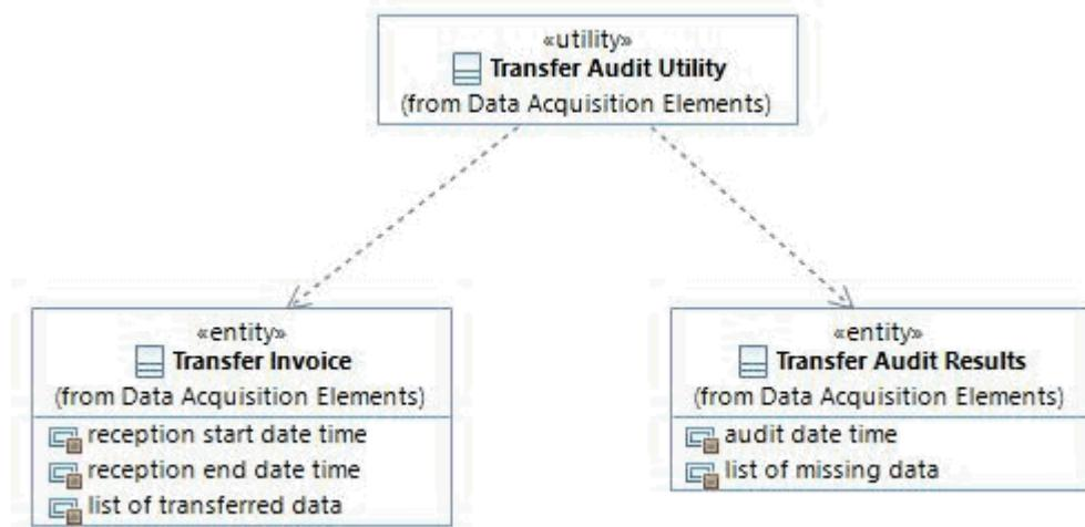
This class diagram depicts the Transfer Audit Utility class and related classes. The Transfer Audit Utility is used by the Transfer Control instance on the receiving Data Acquisition Partition to read the Transfer Invoice and produce the Transfer Audit Results.
