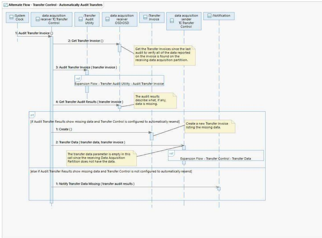
This flow is performed only on the receiving Data Acquisition Partition. The Transfer Control instance on the receiving Data Acquisition Partition periodically audits data frames transferred from the sending Data Acquisition Partition against the Transfer Invoice to verify the data was successfully transferred to the receiving Data Acquisition Partition and stored in the OSD.
