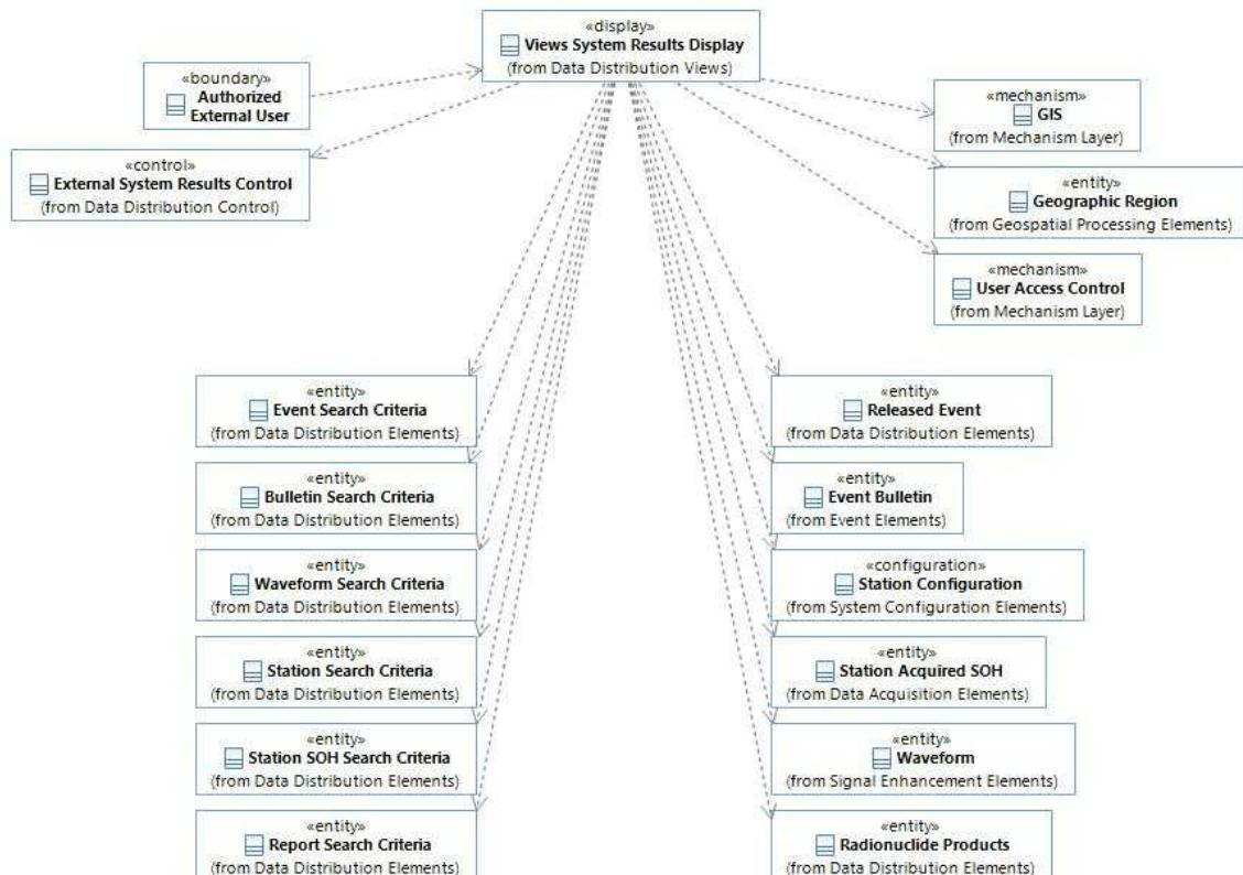
This diagram shows the Views System Results Display class and related classes. The display requests results from External System Results Control using the various "search criteria" classes and displays the results in both tabular and GIS form. The display uses the GIS mechanism to display the results on a map. The display uses the User Access Control mechanism to validate
