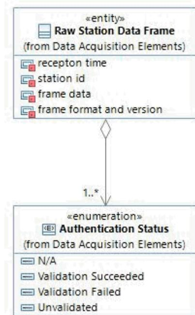
This diagram depicts the Raw Station Data Frame class and related classes. Frame data within the Raw Station Data Frame is stored in the System format. To facilitate possible migration to future formats, each Raw Station Data Frame keeps track of its format and version. Each frame may optionally have a digital signature. The System attempts to validate signed frames. Frames without digital signatures have Authentication Status of "N/A".
