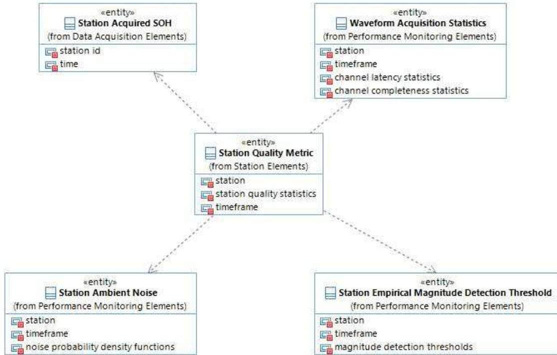
This diagram shows the classes representing Station state-of-health (SOH) including the SOH information acquired from Stations, acquisition statistics, ambient noise, empirical magnitude detection thresholds, and quality metrics.
