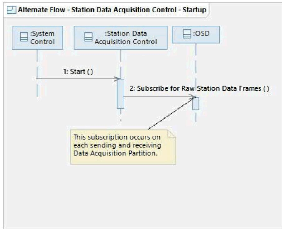
This flow illustrates how the Station Data Acquisition Control subscribes for OSD callbacks on startup, which allows it to respond to and process Raw Station Data Frames when they are stored in the OSD. This flow occurs on each Data Acquisition Partition.
