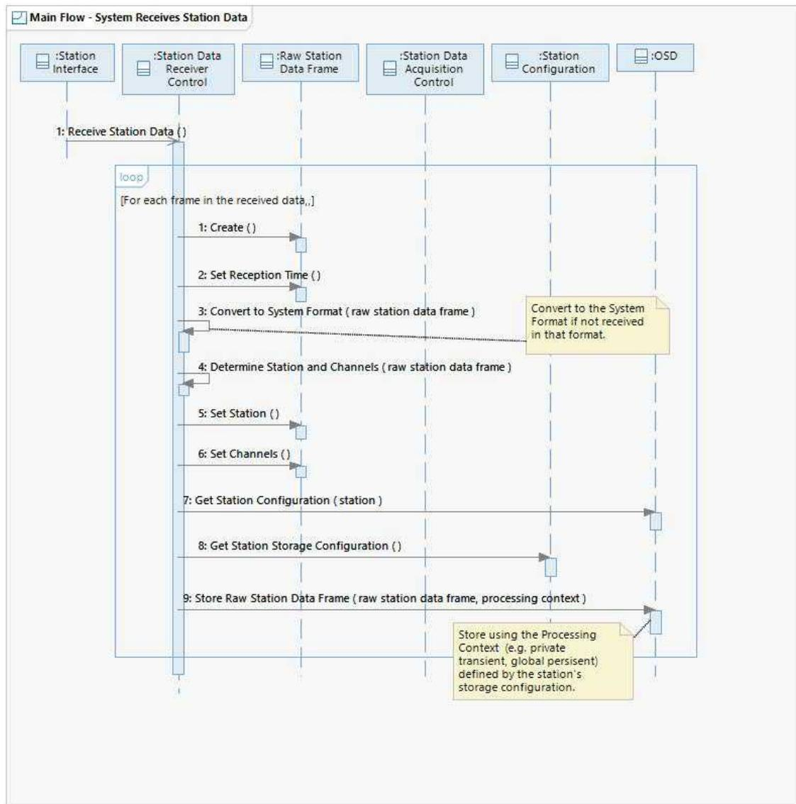
This flow shows Station Data Receiver Control receiving and formatting data frames from seismic, hydroacoustic, and infrasound stations.
