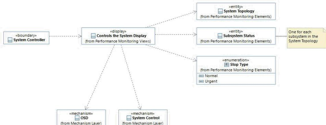
This diagram shows the "Controls the System Display" and related classes. The display is used by the System Controller to control the system and displays System Topology (obtained via OSD subscription) and Subsystem Status (obtained via System Control).
