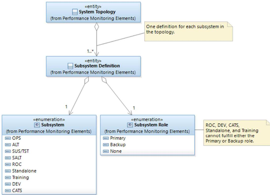
This diagram shows the System Topology class and related classes. System Topology defines a group of related subsystems and the Primary/Backup mission roles currently designated for the subsystems.
