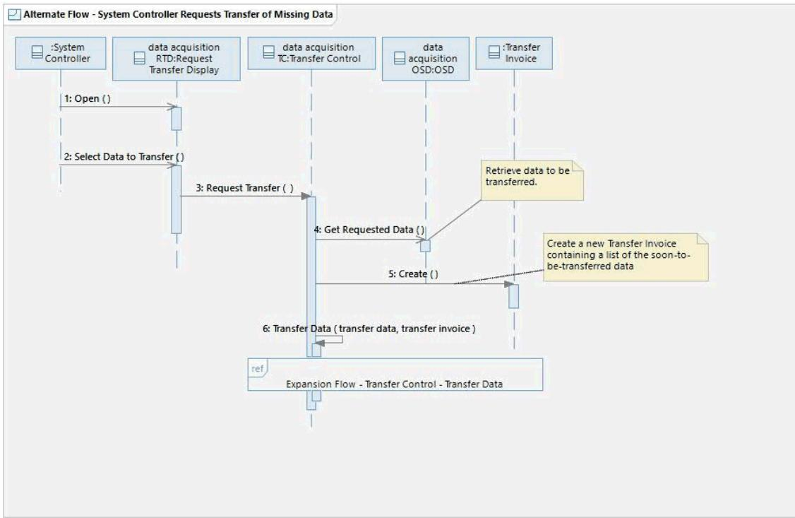
This flow is performed only on the sending Data Acquisition Partition. The System Controller uses the Request Transfer Display to request transfer of missing data from the sending Data Acquisition Partition to the receiving Data Acquisition Partition.
