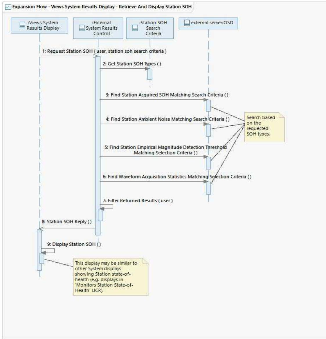
This flow shows how the Views System Results Display uses the External System Results Control to request various types of Station SOH for display to the Authorized User.
