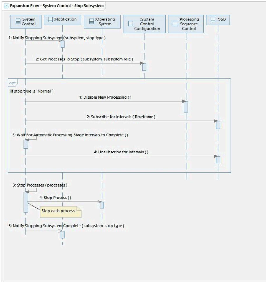
This flow shows how the System Control mechanism stops a subsystem. The subsystem, current subsystem role (Primary, Backup, None), and stop type (Normal or Urgent) are inputs to this flow.
