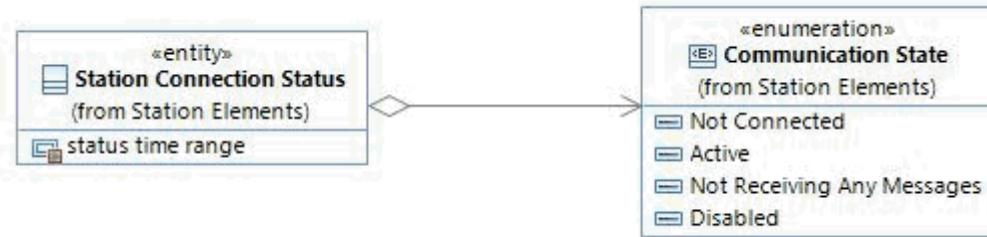
This diagram shows the Station Connection Status class, which is maintained by Station Receiver Control for each station connection.
