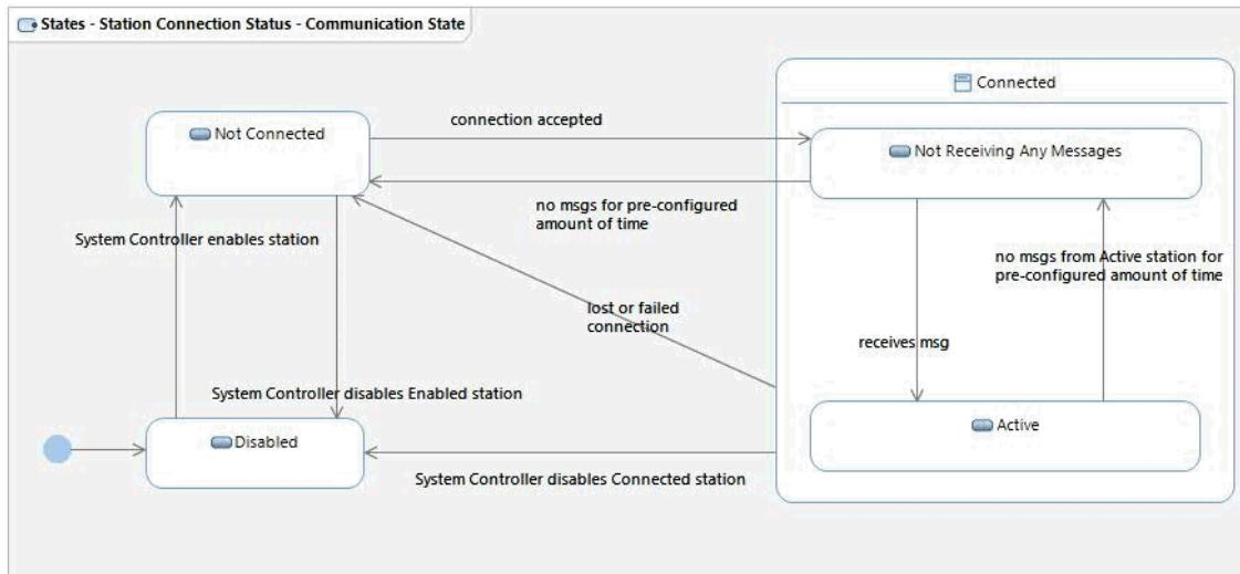
This diagram shows the state transitions for the states defined in the "Communication State" enumeration. These states are maintained by Station Data Receiver Control for individual stations. The System Maintainer configures the timeouts for the state transitions which occur when no messages have been received for a pre-configured amount of time.
