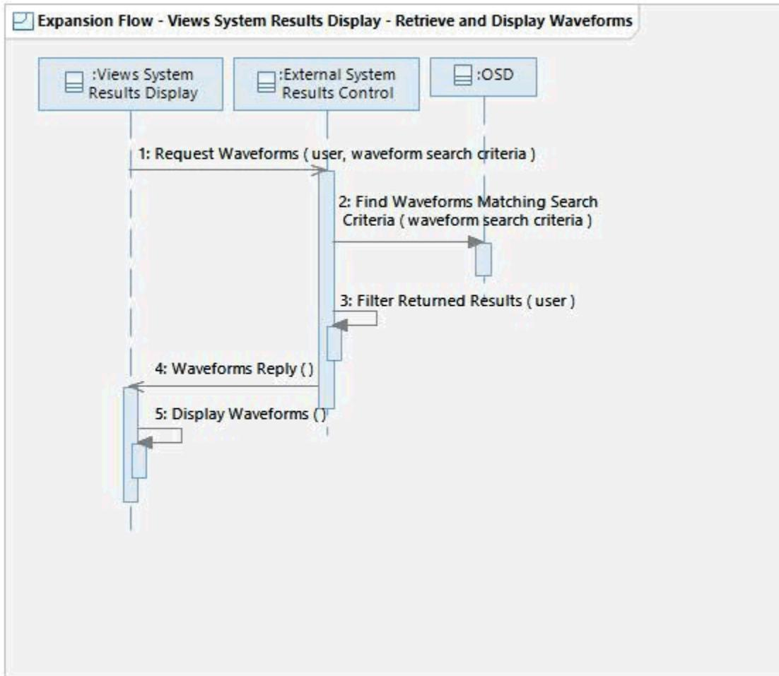
This flow shows how the Views System Results Display uses the External System Results Control to request Waveforms for display to the Authorized External User.
