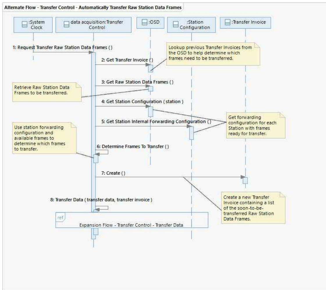
This flow is only performed on the sending Data Acquisition Partition. The Transfer Control class periodically transfers Raw Station Data Frames from the sending Data Acquisition Partition to the receiving Data Acquisition Partition.
