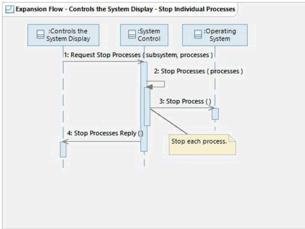
This flow shows how the Controls the System Display stops individual processes. This flow receives the process to stop and the Subsystem where the process is running. The System Controller selects these values in the invoking flow. This flow supports the case where a process is running but not functioning properly (e.g. non-responsive) and needs to be restarted.
