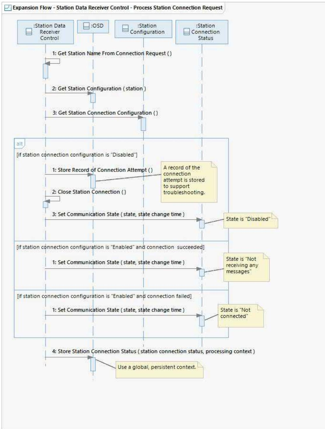
This flow describes how the Station Data Receiver Control processes a station connection
