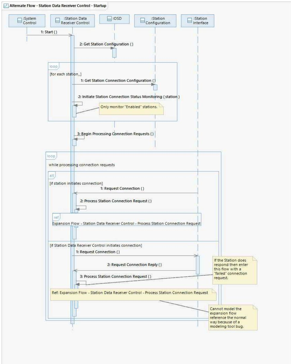
This flow describes how the Station Data Receiver Control initializes at startup. Station Data Receiver Control opens, listens for incoming station connection requests, and processes requested station connections. Station Data Receiver Control also monitors the connection status of enabled stations (see 'States - Station Connection Status - Communication State' for the possible connection states).
