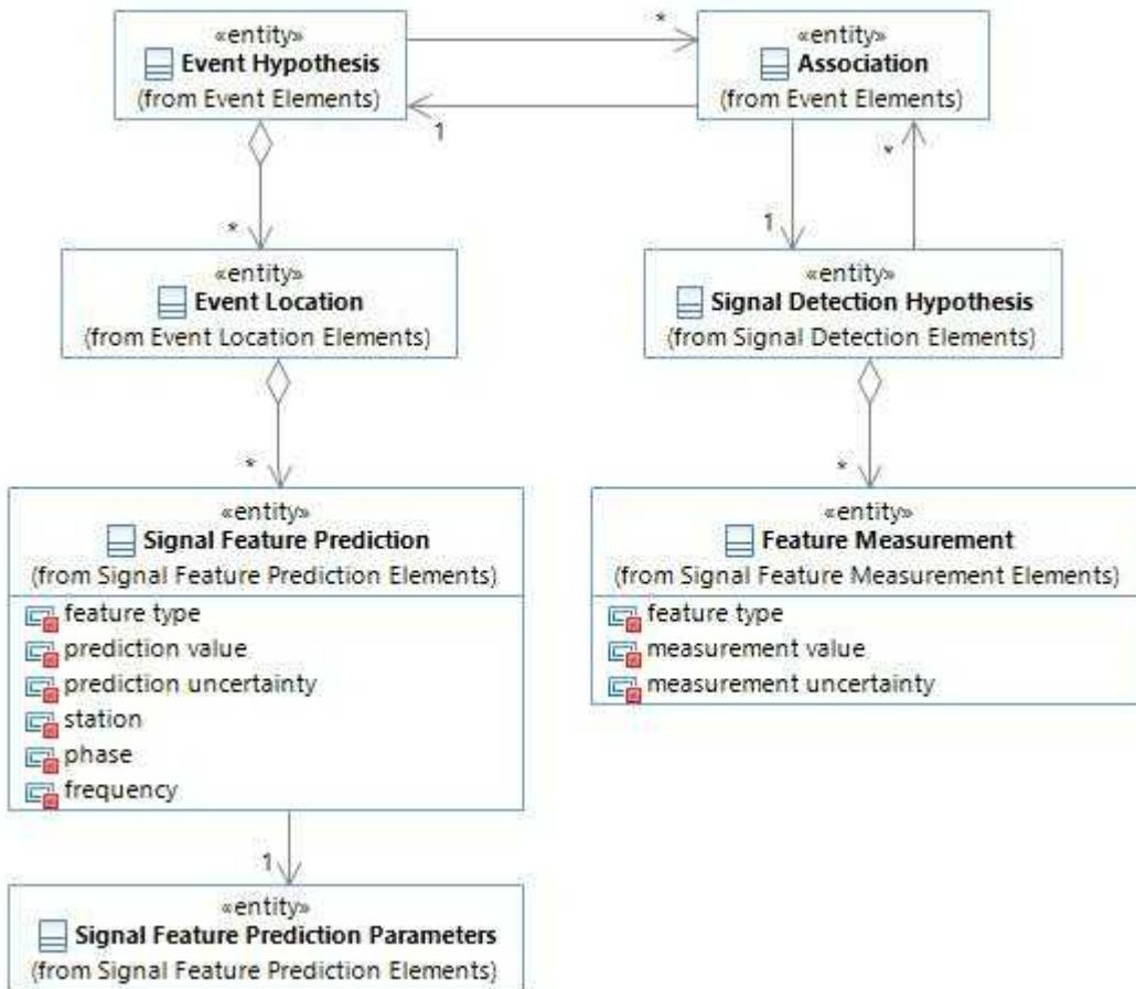
This diagram shows how the Signal Feature Prediction and Signal Feature Prediction Parameters classes relate to the Event Hypothesis class via the Event Location class. Tracing associations backwards from Signal Feature Prediction to Feature Measurement show the relationship between corresponding prediction and a measurement values. Using this type of a relationship or a more direct relationship between these classes is an implementation detail.
