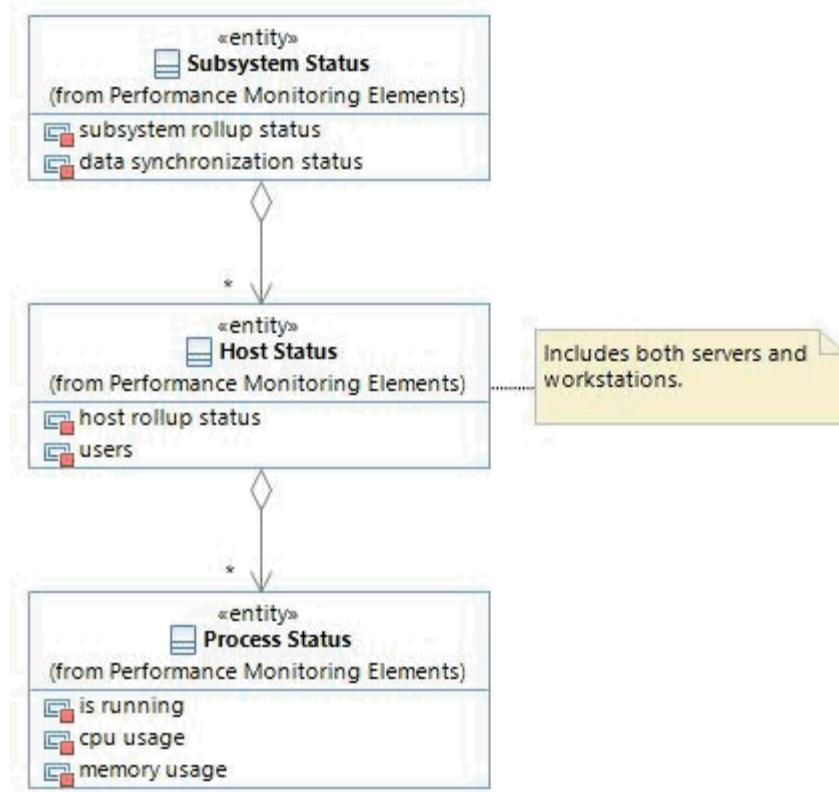
This class shows the Subsystem Status class and related classes. Subsystem Status is determined by System Control.
