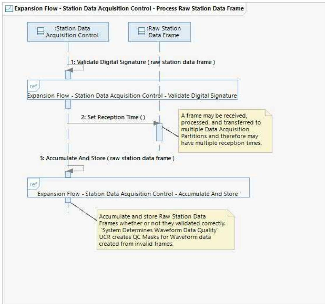
This flow describes how the Station Data Acquisition Control processes station data.
