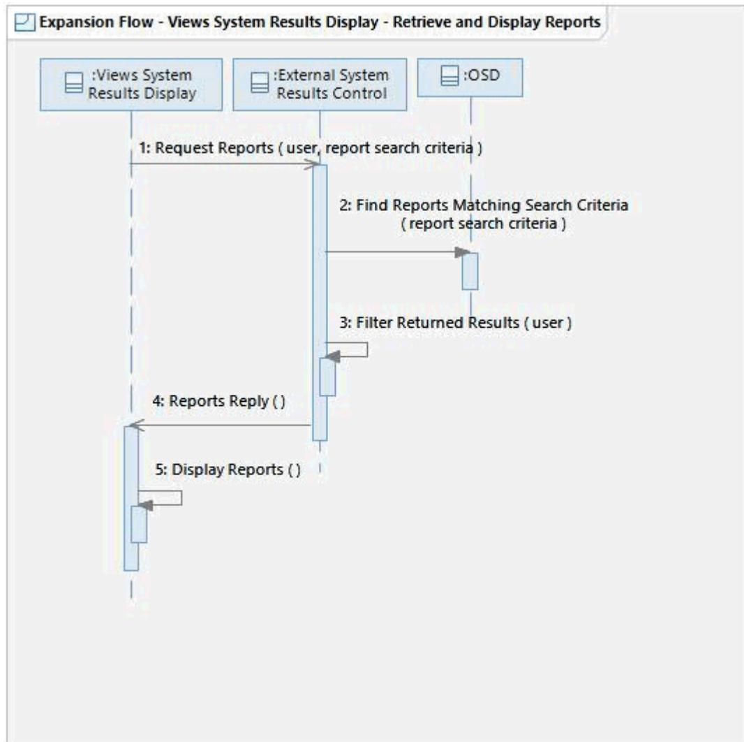
This flow shows how the Views System Results Display uses the External System Results Control to request Reports for display to the Authorized External User.
