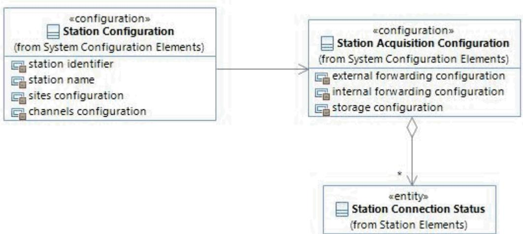
This diagram shows the Station Configuration class and related classes. Station Configuration information is configured by the System Controller (see "Controls Data Acquisition" and "Configures Station Usage" UCRs).
