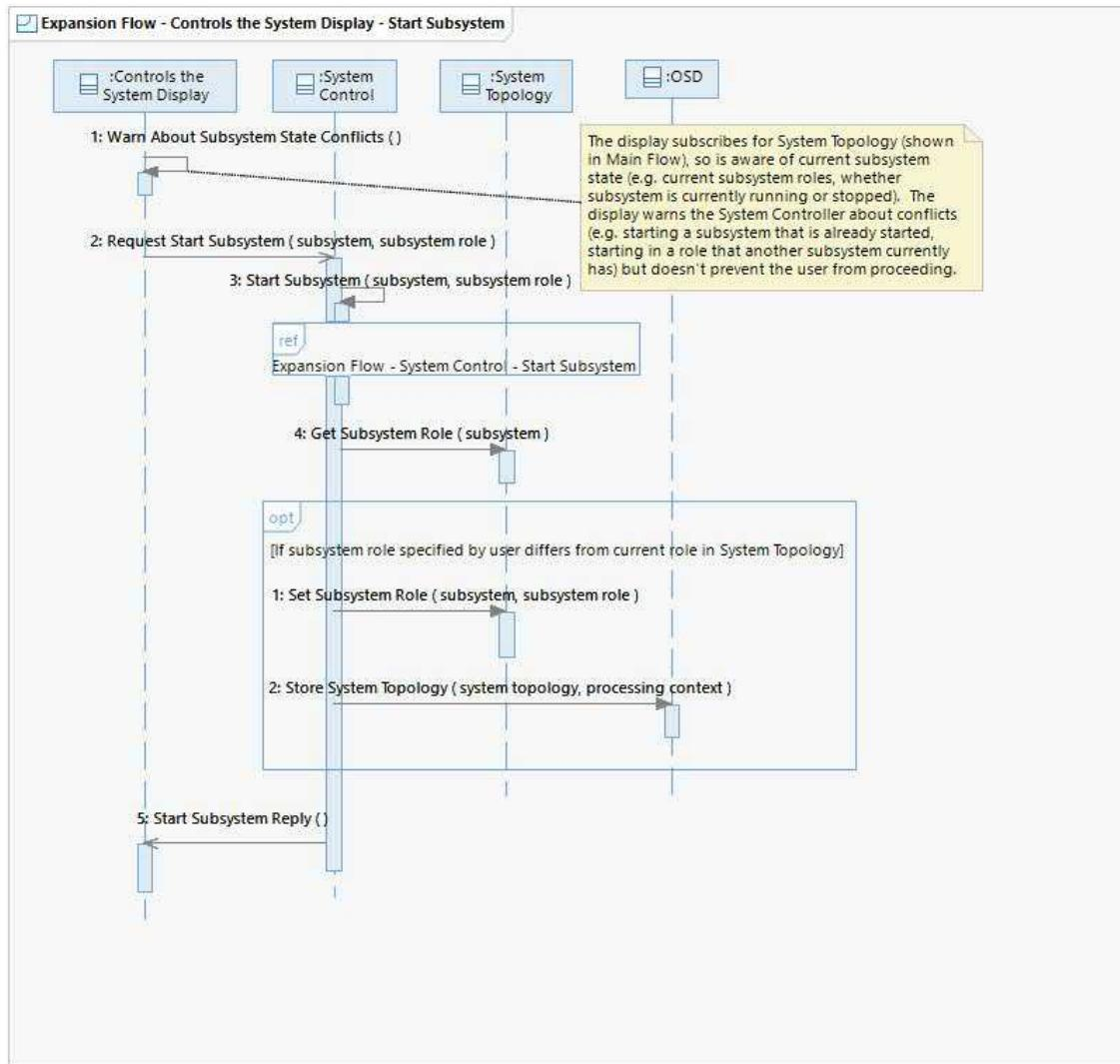
This flow shows how the Controls the System Display starts a subsystem. This flow receives the subsystem to start and the role for the subsystem to start up as (Primary, Backup, or None). The System Controller selects these values in the invoking flow. The display warns the System Controller and updates the System Topology if the specified role differs from the current System Topology.
