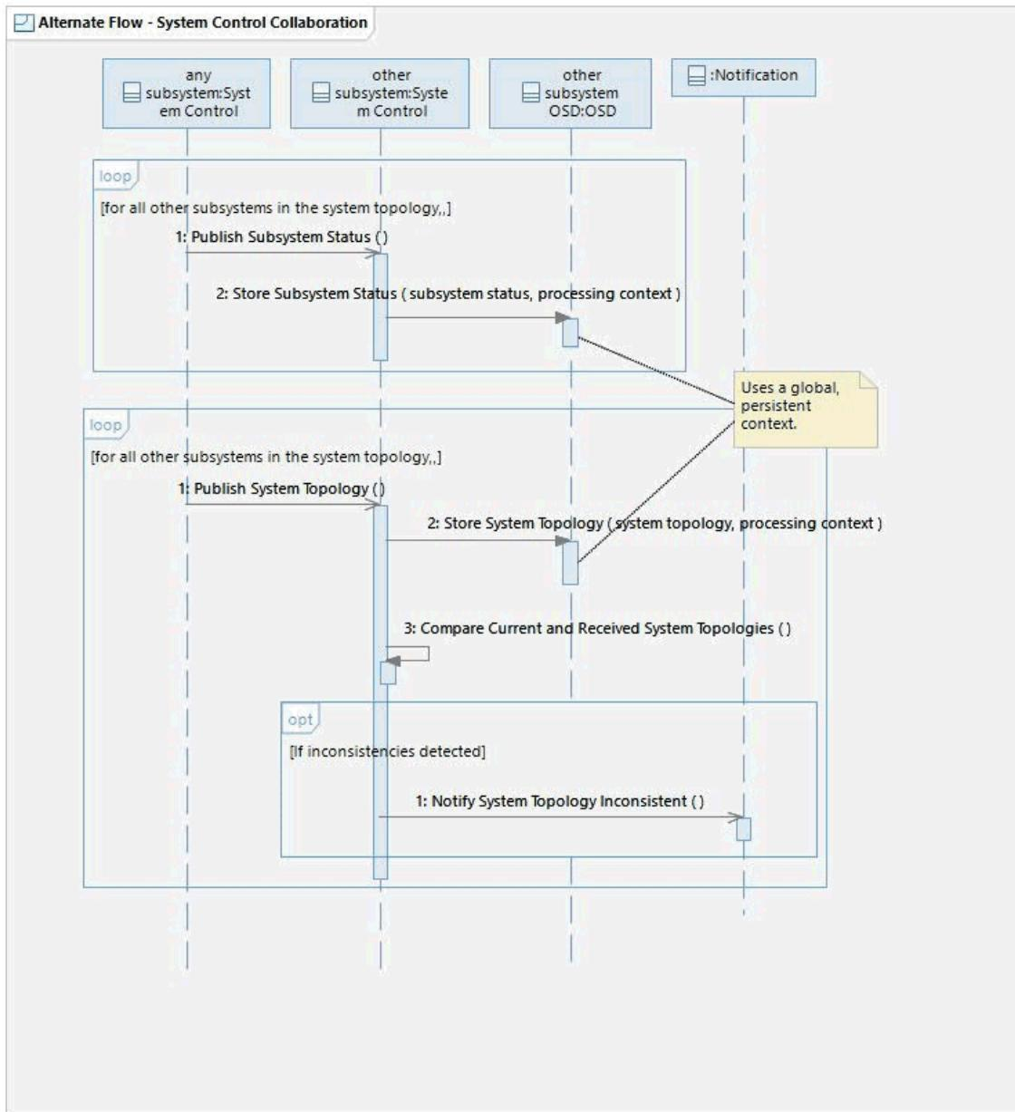
This flow shows how each subsystem in a system topology shares its Subsystem Status and System Topology with the other subsystems in the system topology. Each instance publishes its own Subsystem Status and System Topology and subscribes for the Subsystem Status and System Topology from the other subsystems. The System Controller is notified of inconsistencies between subsystems (e.g. if subsystems have different notions of the current System Topology).
