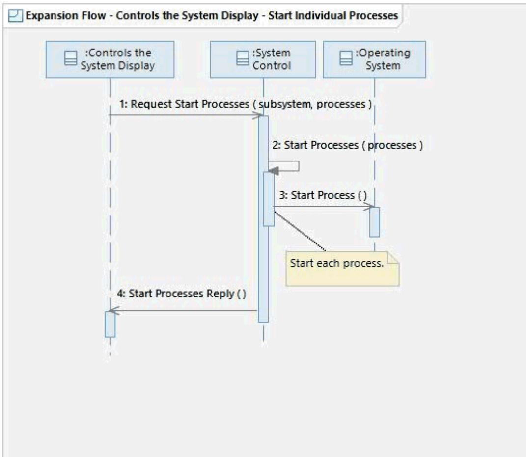
This flow shows how the Controls the System Display starts individual processes. This flow receives the processes to start and the Subsystem where the process should run. The System Controller selects these values in the invoking flow. This flow supports the case where a process that is expected to be running has crashed and needs to be restarted.
