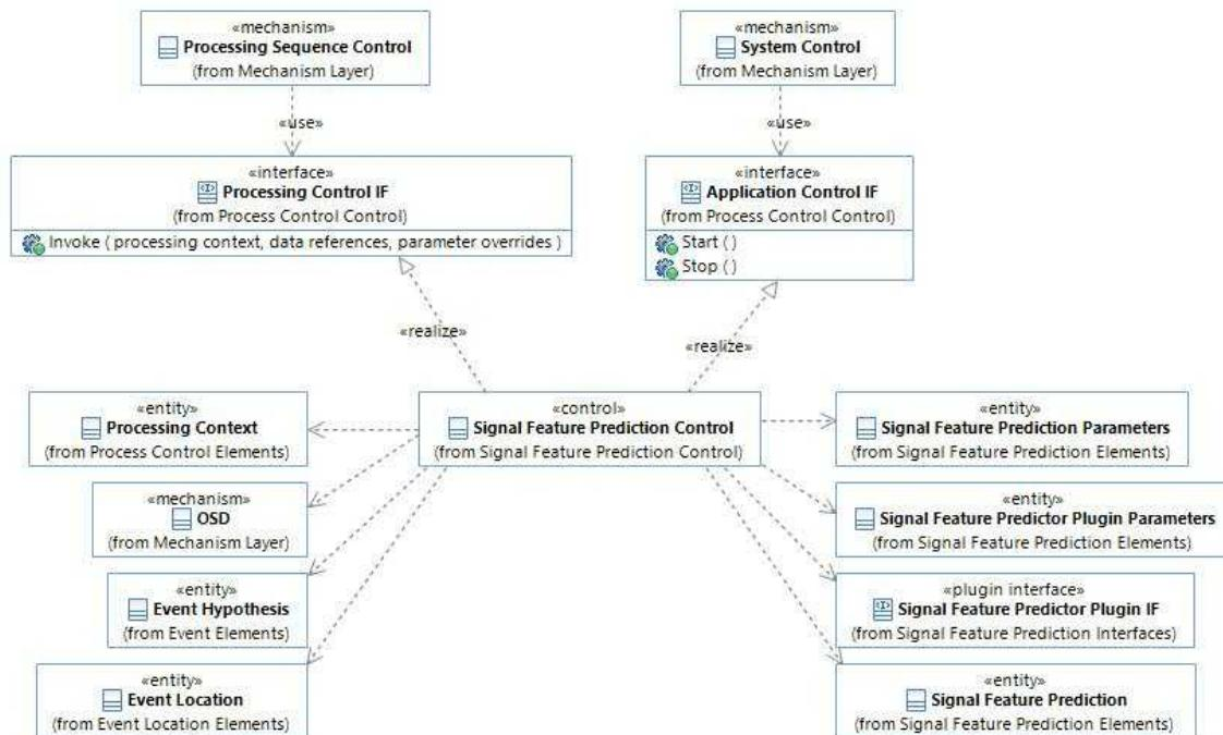
This diagram shows the Signal Feature Predictor Control class and related classes. The Control class invokes a Signal Feature Predictor Plugin via the plugin interface to compute Signal Feature Predictions. The prediction is based on a particular Event Location and a particular station location. The Control class associates the prediction to the Event Location and stores the predictions in the OSD.
