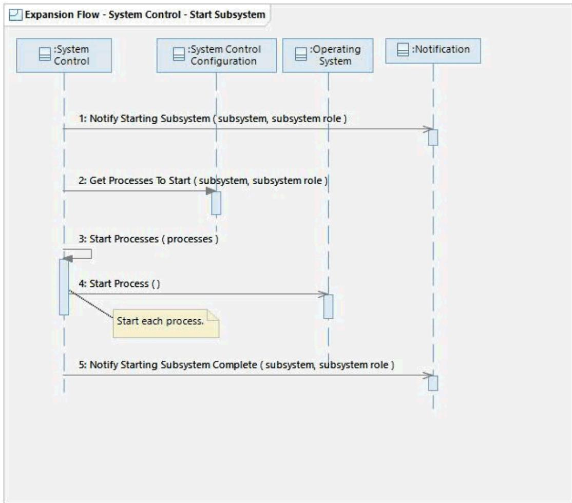
This flow shows how the System Control mechanism starts a subsystem. The subsystem and its current subsystem role (Primary, Backup, or None) are inputs to this flow.
