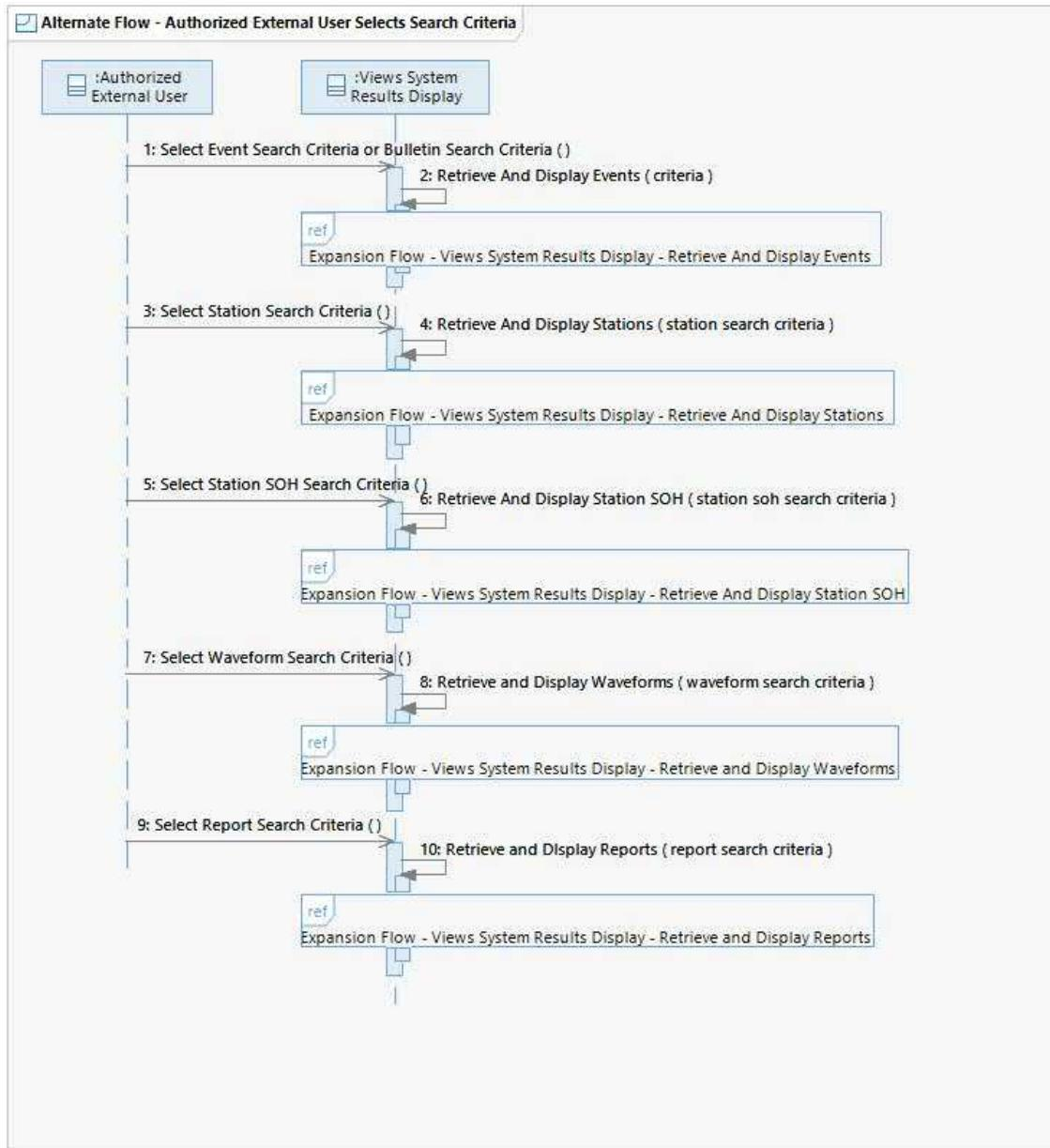
This flow shows how the Authorized External User can tailor the information displayed by Views System Results Display by selecting the search criteria External System Results Control uses to query the OSD. The Authorized External User may also subscribe to regularly receive updated System results matching the search criteria entered in this flow (e.g. subscribe based on station, event location, event azimuth from station, SNR, etc.). See 'Requests System Data' UCR for details.
