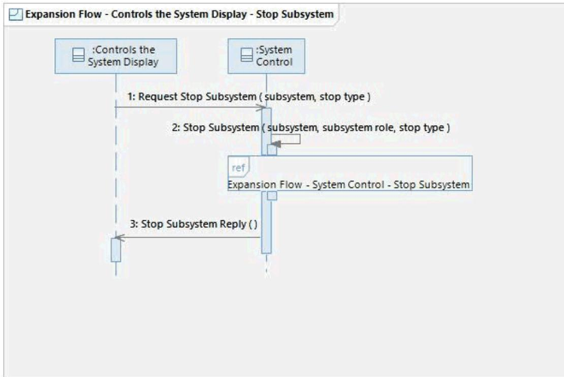
This flow shows how the Controls the System Display stops a subsystem. This flow receives the subsystem to stop and the stop type (Normal or Urgent). The System Controller selects these values in the invoking flow. The display requests the System Control mechanism to stop the subsystem. Note that stopping a subsystem does not affect the subsystem's role in the System Topology (Primary, Backup, or None).
