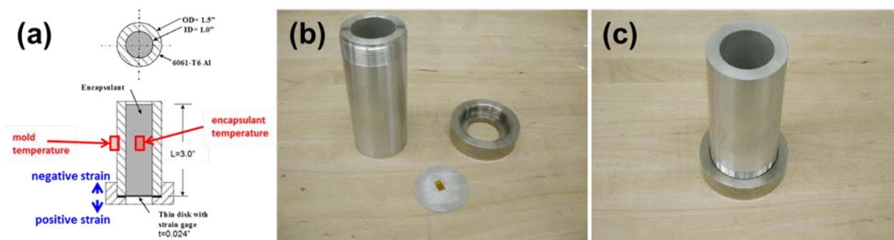
Figure 3. Thin-disk-on-cylinder (a) schematic, (b) individual parts and (c) assembled structure.
