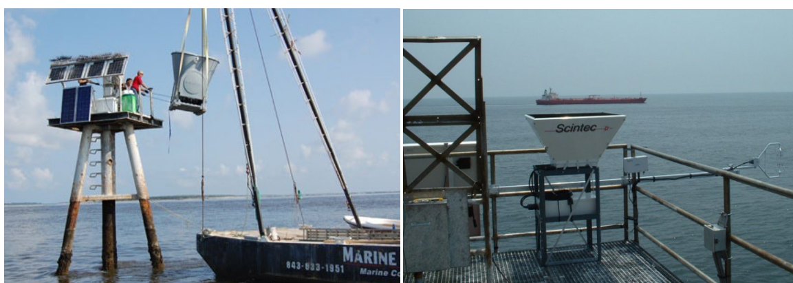
Figure 4.6 US Metocean Monitoring Deployments on Existing Platforms: Sodar deployment on a US Coast Guard Platform in South Carolina 4 (left), and Portions of the metocean monitoring package installed on the (now decommissioned) Ambrose Light Station in NY Harbor (right).
