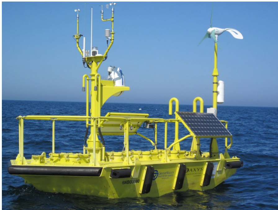
Figure 4.4 Buoy-Based Lidar System. (Source: AXYS, 2014)
