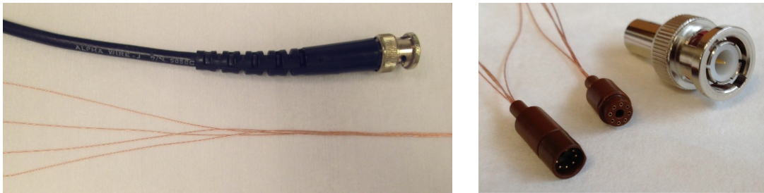
Figure 3. Left: A cable bundle with a BNC cable for comparison. Right: A male-female signal connector pair, with a BNC connector for comparison.
