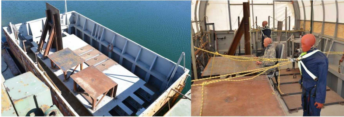
Figure 3: Floating Shock Platform test setup
