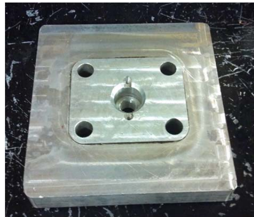
Figure 3.6: Fabricated cylinder head for low temperature combustion study.
