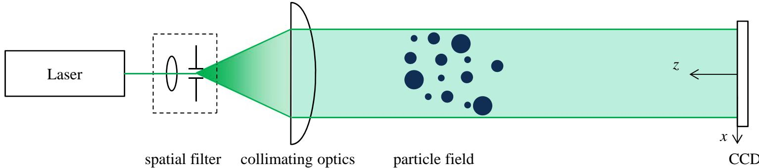
Holographic plate and wet-chemical processing replaced with digital sensor
