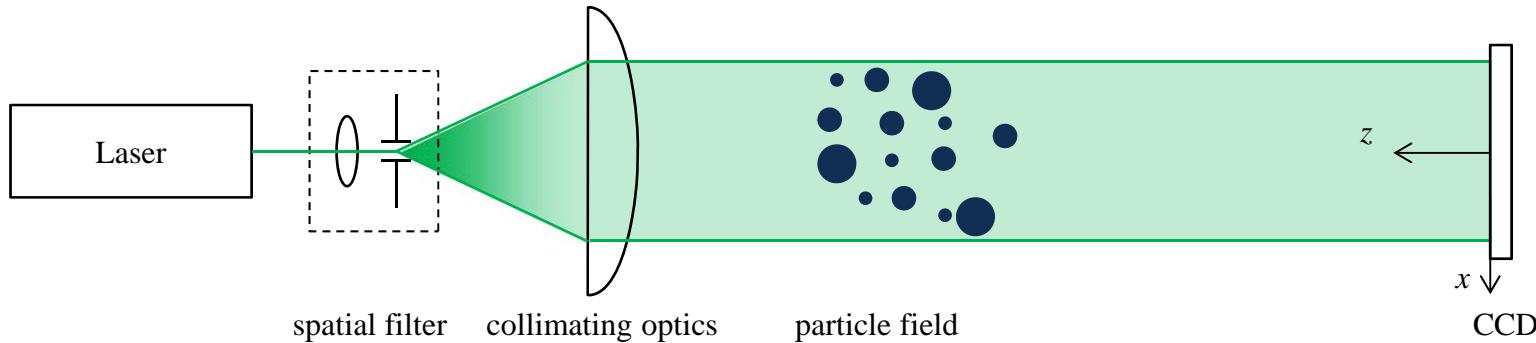
Hologram is the combination of object and reference waves:  $h = |E_o + E_r|^2$
