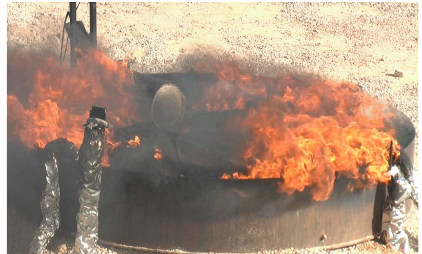
Rubble fire involving 900 lbs. of composite material and 320 gal. of jet fuel
