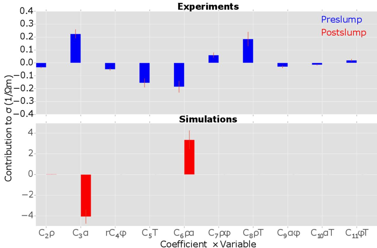
Density and particle size distribution are the most significant processing parameters
