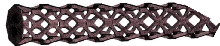
solution for a bar in pure torsion resembles a cholla cactus
