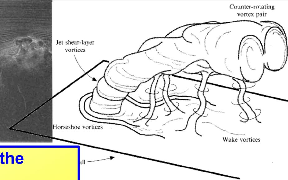
**Shear layer vortices are important to the CVP development in the near-field.**
