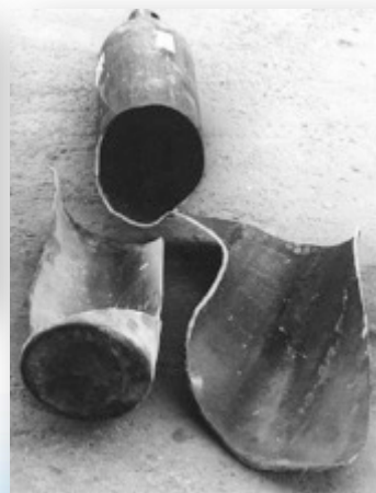
example of embrittlement failure from the 1970's
